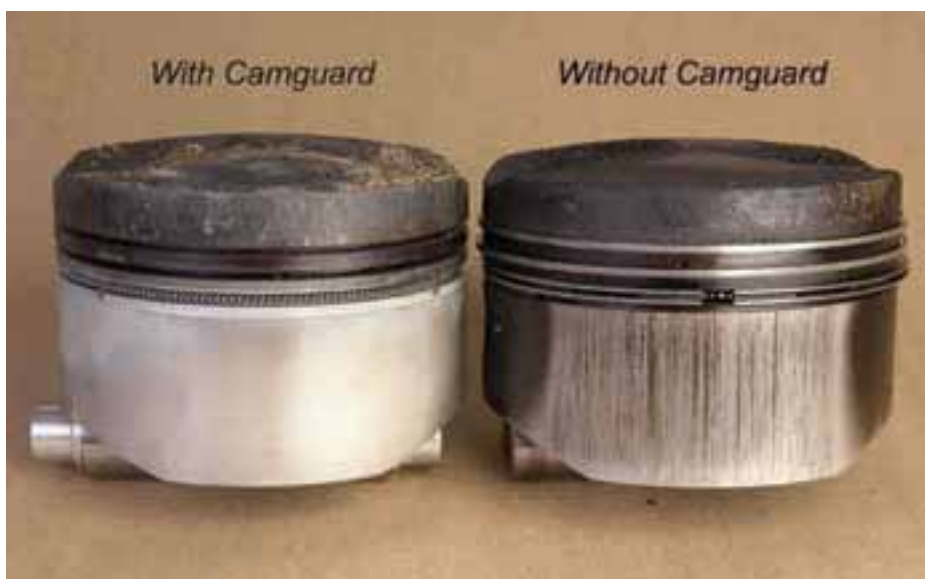
Comparable pistons; the left one used Cam Guard.
