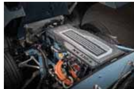
The battery pack needs cooling, hence familiar-looking radiator and piping.
