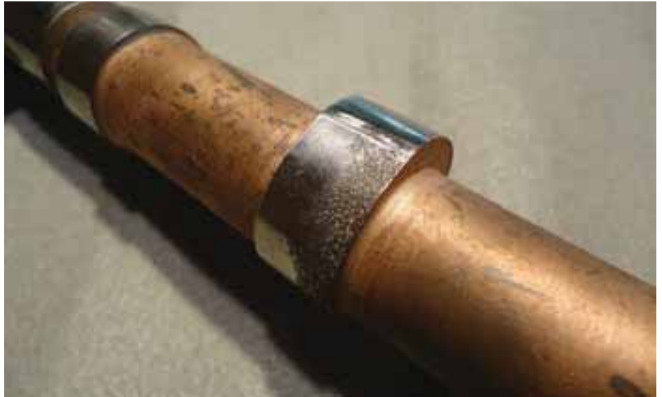
A flattened non-Jaguar cam. Jaguar material is very durable but could this happen?
