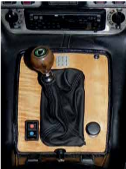
Discrete two-way (hotter or colder) rocker control bottom left is a repurposed power lock switch. The fan switch is still used.
