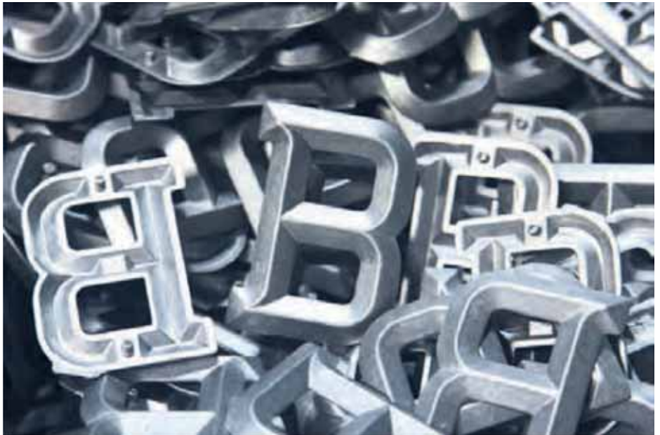
The best are used, the rest are rejected. Pressure die-casting gives accurate sizing, including on the fixing studs.
