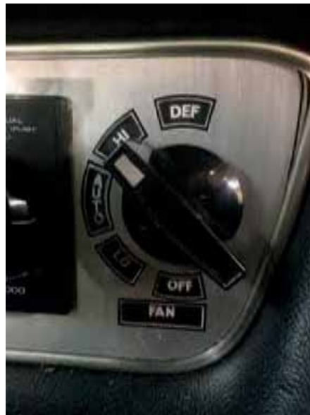
The variable fan switch is used as normal, even if the temperature one is bypassed.
