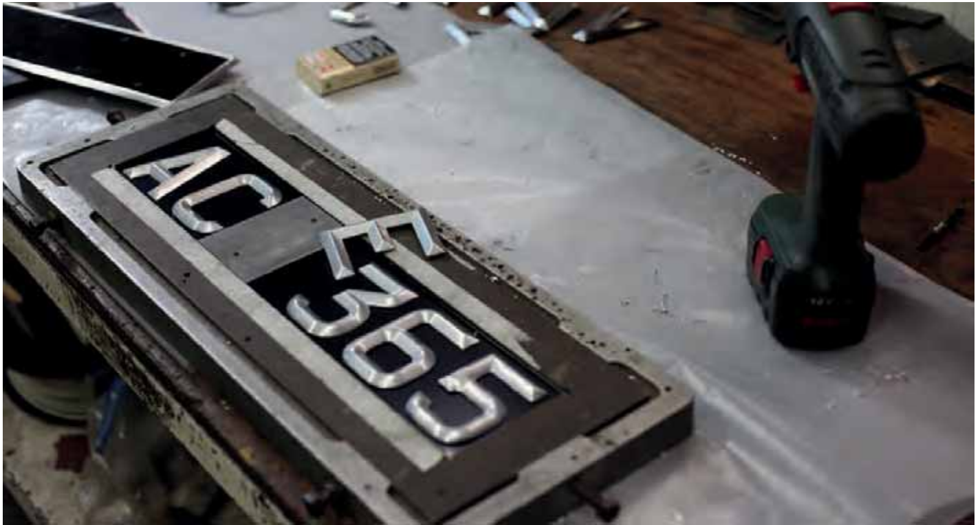
A jig frame and templates for each letter ensure accurate drilling into the background plate.
