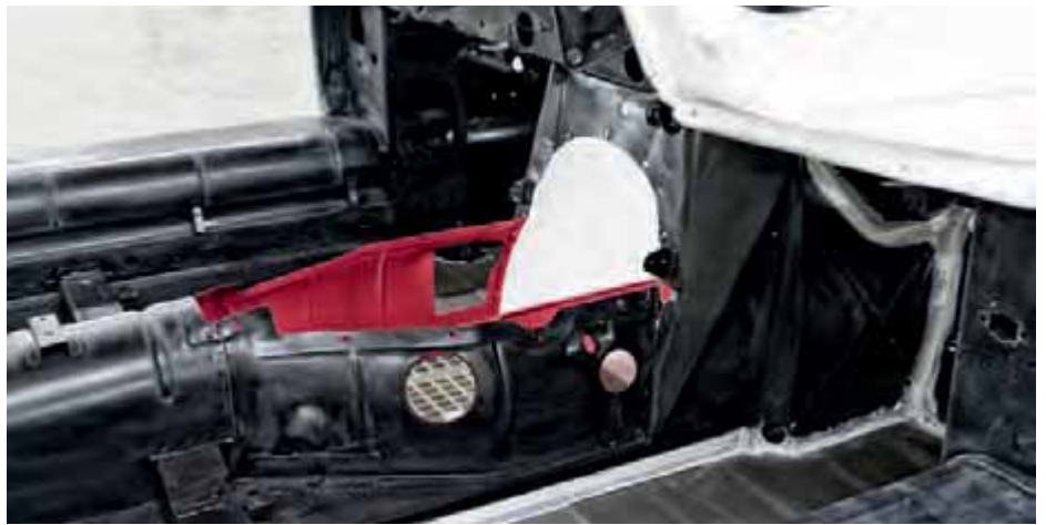
Fresh metal prep and seam sealer.
