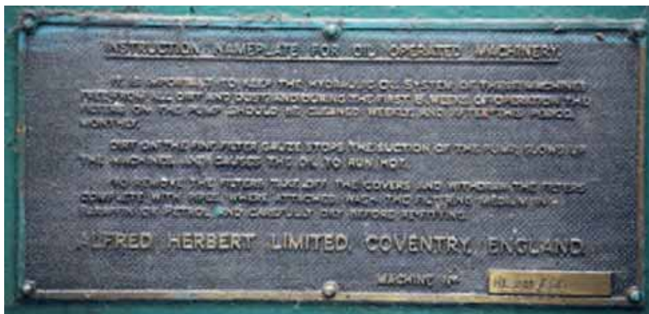
Manuals rot, or burn or disappear. The instructions for the Herbert are, appropriately, a die cast plate riveted to the machine.
