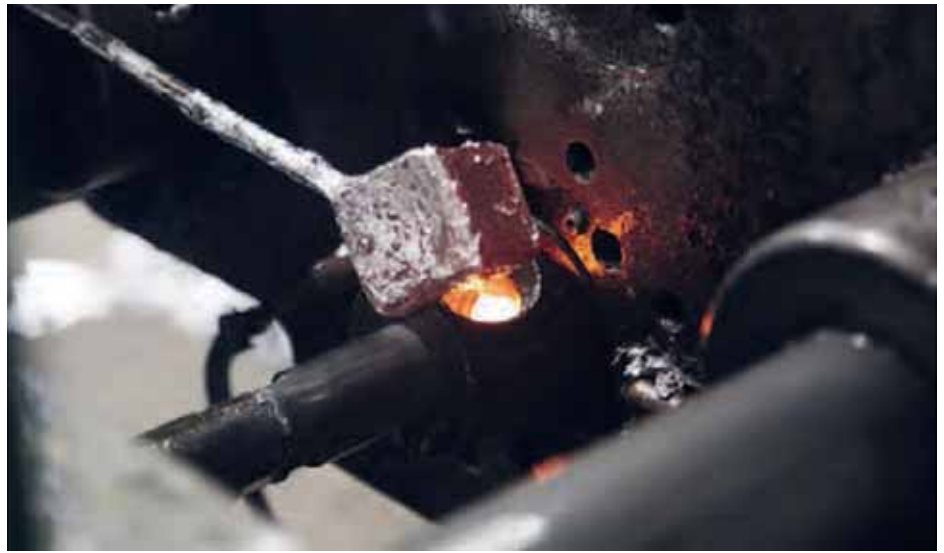
Spooning the alloy into the chamber before squeezing into the dies.
