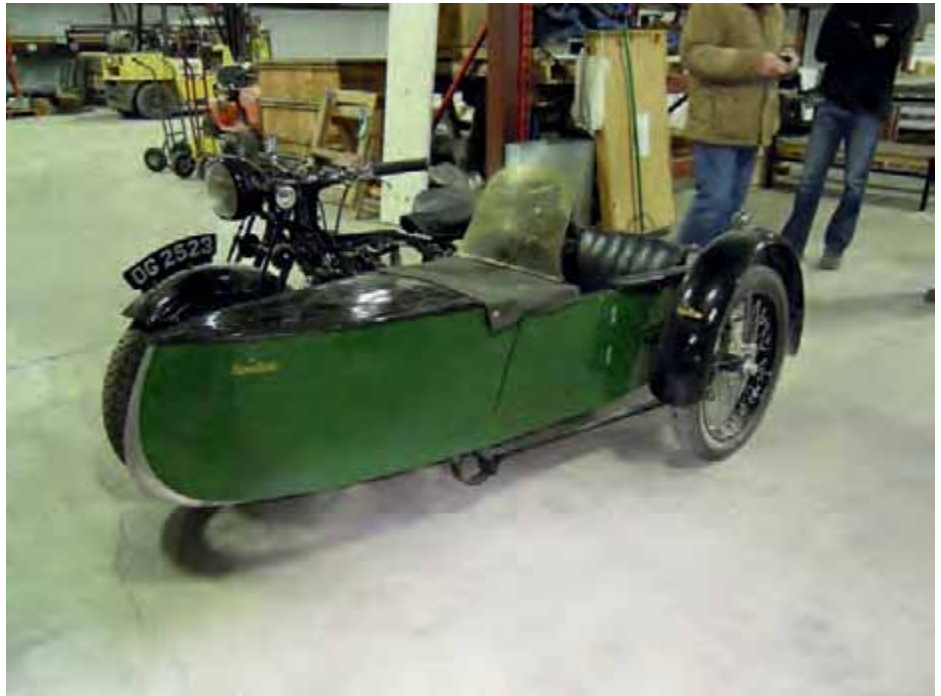
Very pretty boat-style single seat sports sidecar, hitched to the left (UK) side of a 500 cc workhorse BSA OHV Sloper.
