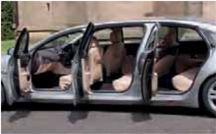
No need to move down the bus with doors provided for all three X350 seat rows.
