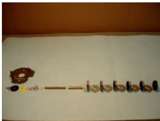
Lift out the tumblers and separate all the pieces for cleaning use mild soap and water using a toothbrush.
