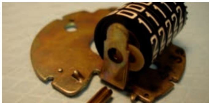
Slide the tumbler stack back into the bracket and insert one of the two white plastic locking collars and line it up with the hole.
