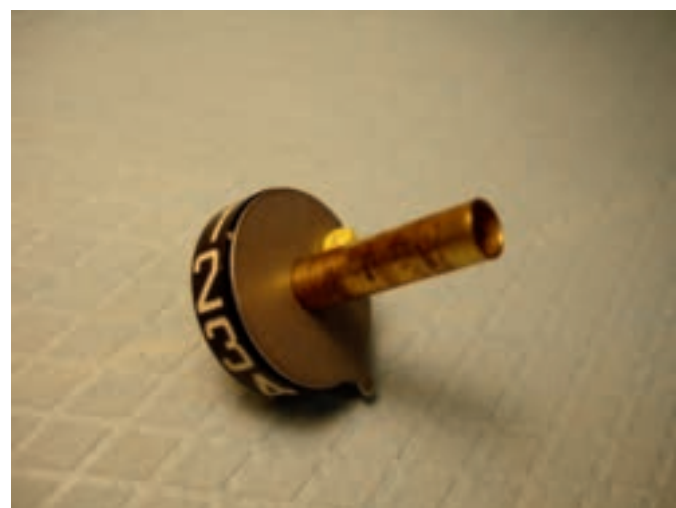
Reassembly sequence, Tumbler then indexer and guide.
