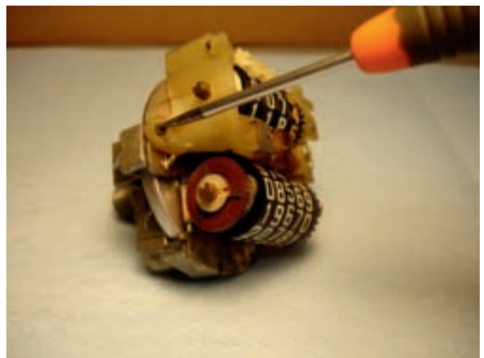
Remove the screws to separate the odometer from the speedometer base.
