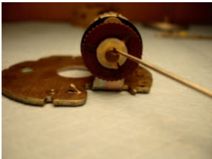
Remove the white plastic locking clip.
