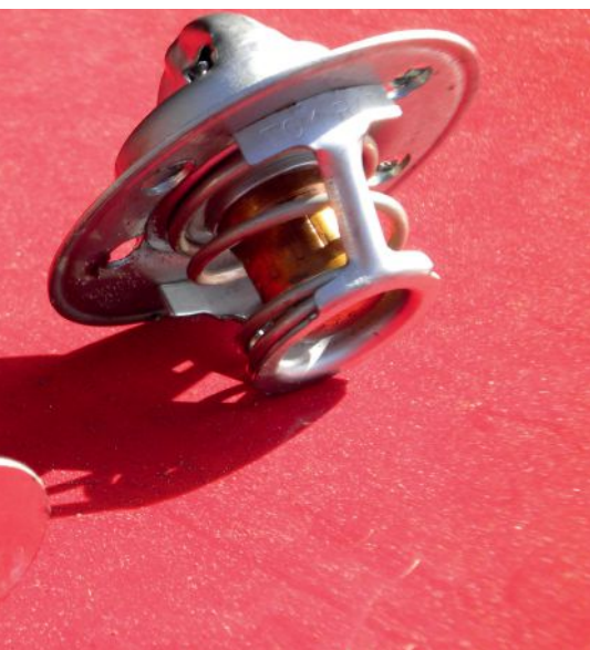
right leaves the bypass open and spoils cooling.
