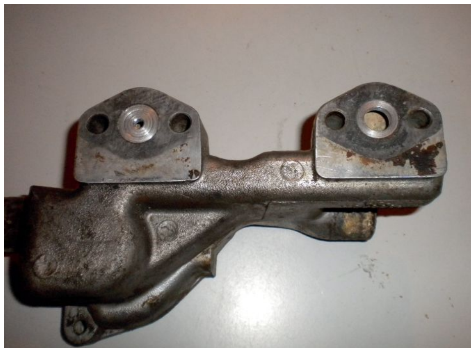
Differential-sized restrictors shown in situ.
