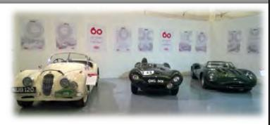
The one and only XJ13 from 1966. Designed to be a Le Mans competitor to succeed the D-type, the XJ13 was fitted with a quad cam 5.0 litre V12 engine to give it a top speed approaching 200mph. Sadly the rules were changed before it was completed, limiting Le Mans cars to engine capacities not exceeding 3.0 litres. This left the XJ13 sidelined and this is the only complete surviving example.
