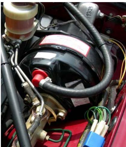
ABS has no large vacuum servo, as boost is hydraulic.
