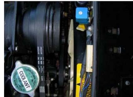
**RADIATOR CAP:** To 1982 one on the header tank. 1982 two total with one chained to header tank, made by AC, turn down tight remove when cold, and one on the fill tube at the middle front of the engine with blue on white with black lettering "Coolant" circular label. (see photo above) 1984 3.6 has one cap on the left front fender header tank made by AC with attaching chain. 1989 header tank chain deleted.
