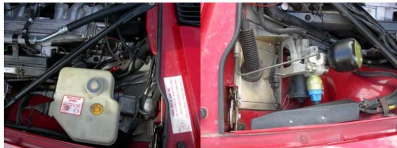
1976 to 1988 Master cylinder and vacuum servo
