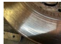
Brake Rotor showing excessive wear. Note: The 33 1/3 Long Playing Record Grooves. Not sure of the tune.
