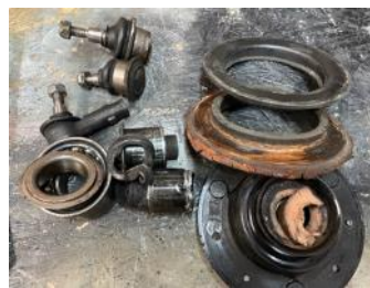
Parts replaced XK8 front end parts. CCW L-R. Upper & lower ball joints, Steering Link, Main Bearing, Lower Bushings, & Shock Mount.
