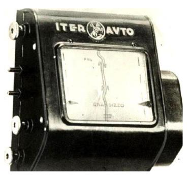
rolling map drivers aid "The 'Iter Avto', the 1930's version of a GPS. Developed by Touring Club Italiano, this device was more like a 'map guidance tool' and came with a set of paper maps. It was tethered to the car's speedometer that kept the scrolling of the map in proportion to the speed of the car.
