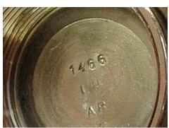
NOS XK wheel spinner wanted new old stock left-hand factory wheel spinner for an XK or E-Type. Jaguar part # C1103. One only. See the images for identification. If it does not have these casting marks on the inside, it is not factory. Anyone? Please! Contact Godfrey Miller, artrageus@shaw.ca, +1 250-415-1158 mobile. Nov 2021
