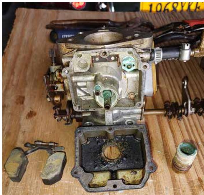
removed the floats, replaced the seat assemblies with new stock ones, re-installed the old floats, adjusted the float height, cleaned the bowls, put everything back together, reinstalled the carbs on the manifold and hooked up the fuel line. Getting the nuts and washers back on the studs was especially frustrating and longer, exacerbated by sweaty, oily fingers on a hot day. Ask me how I know.
