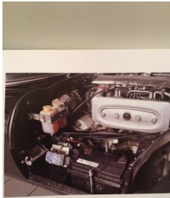
The battery was moved to the right-hand side, and there was a new BUTEC control box mounted just behind it. Above it are the reservoirs for clutch and brake fluid (the latter one of two), and the wiper motor is behind that.
