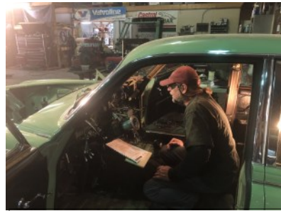
Art meticulously following the workshop manual diagram to install the new wiring.
