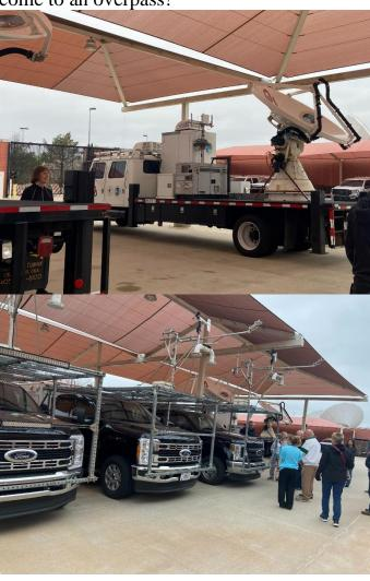
The other trucks are well equipped with cameras and radar – as well as steel grates encasing most of the truck and extending beyond the front ends to protect them from hail damage (somewhat successfully, at least).
