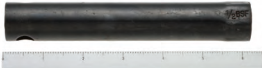
C.179/b Box Spanner, for Spark Plugs
