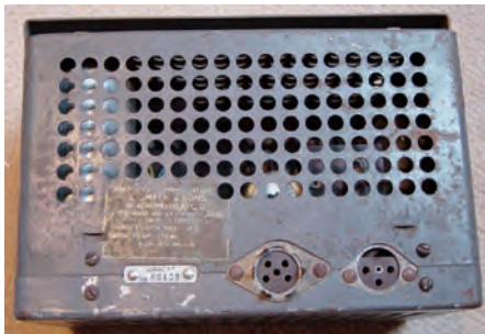
New (round) 5-pin connector type plugs on XB and RB power units. Speaker plug has three pins.
