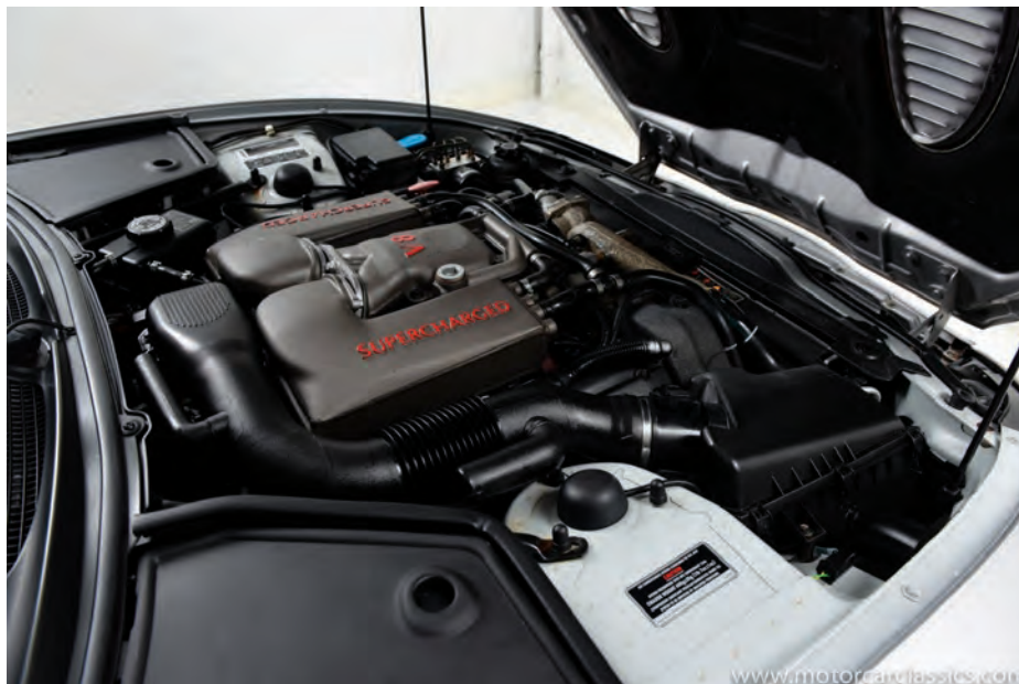
The imposing intercoolers atop the XKR’s already powerful V8. (www.motorcarclassics.com)
