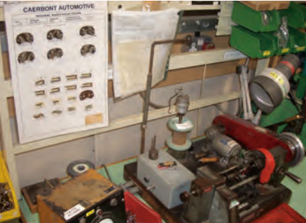
This workstation is for making bi-metal electrical gauges as used on countless classic cars. Note the crib sheet for different types of assembly.
