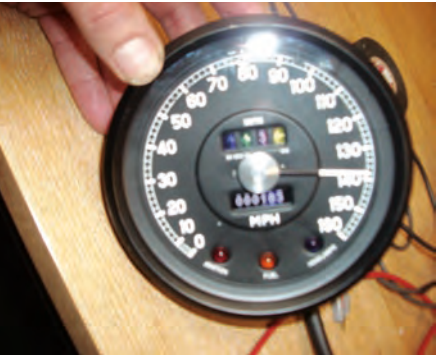
No, your eyes don’t deceive you – the trip digits are different colors and can be programmed at will. An example of targeted R&D that enables Caerbont to deliver a wide range of products without massive, unwieldy infrastructure.
