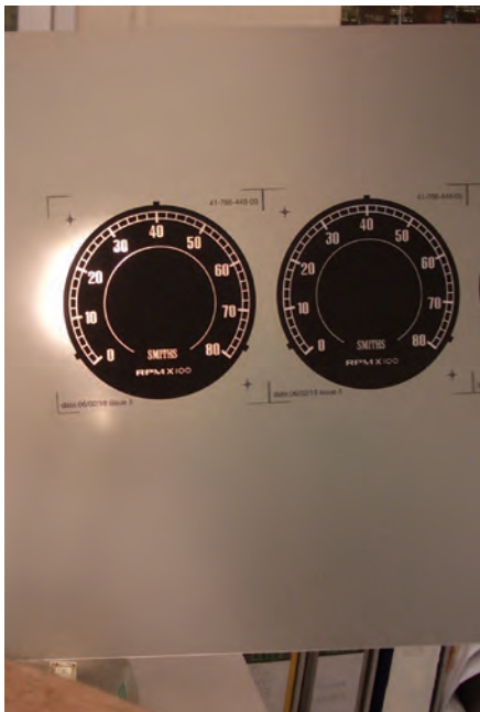
Vastly more effective than period 3W tungsten-filament side illumination, backlit instruments can be made to look standard in daylight whilst being much safer at night.
