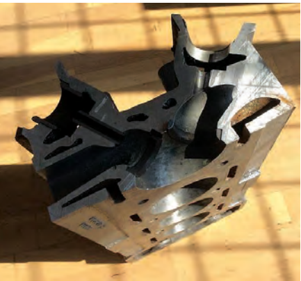
Sectioned Jaguar XK cylinder head – “curved” inlet port on right (© N. Swales).
