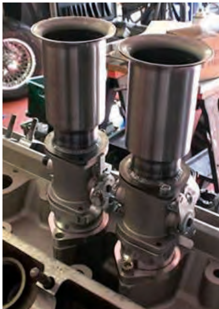
Baily's prototype quad-cam engine showing down-draft arrangement (© N. Swales).
