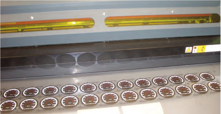
Special equipment prints batches of more modern back-lit instruments.
