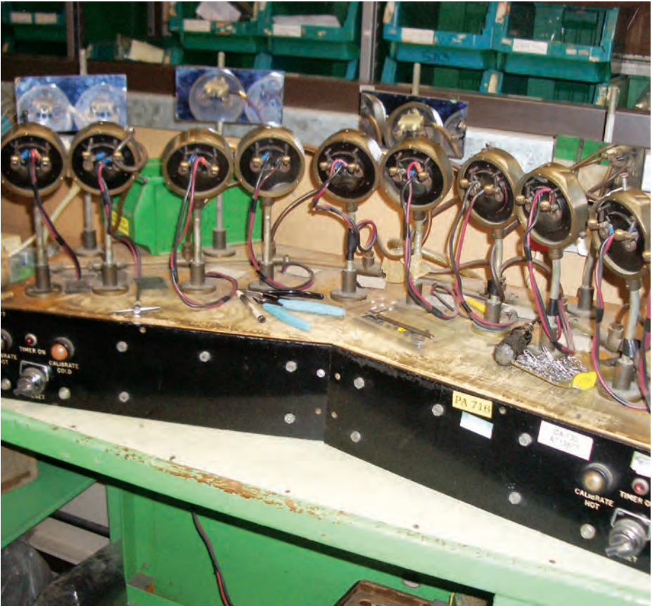
Since basic physics doesn’t change, why should a solidly-constructed calibration bench? This one dates from the WWII era, when lives of soldiers, airmen and sailors depended on good instrumentation. Notice the mirrors behind each pair to avoid parallax error.
