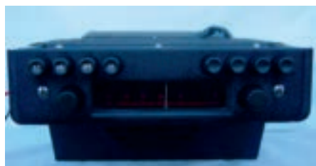
Radiomobile 4012 with medium wave only.
