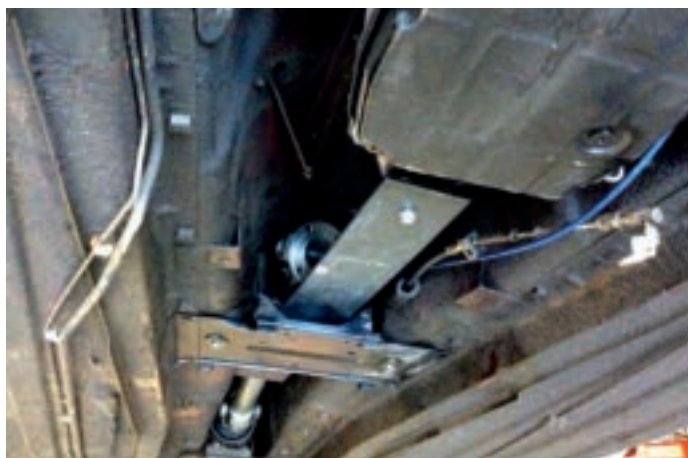
The front driveshaft hook-up is straightforward once length and position are optimized.
