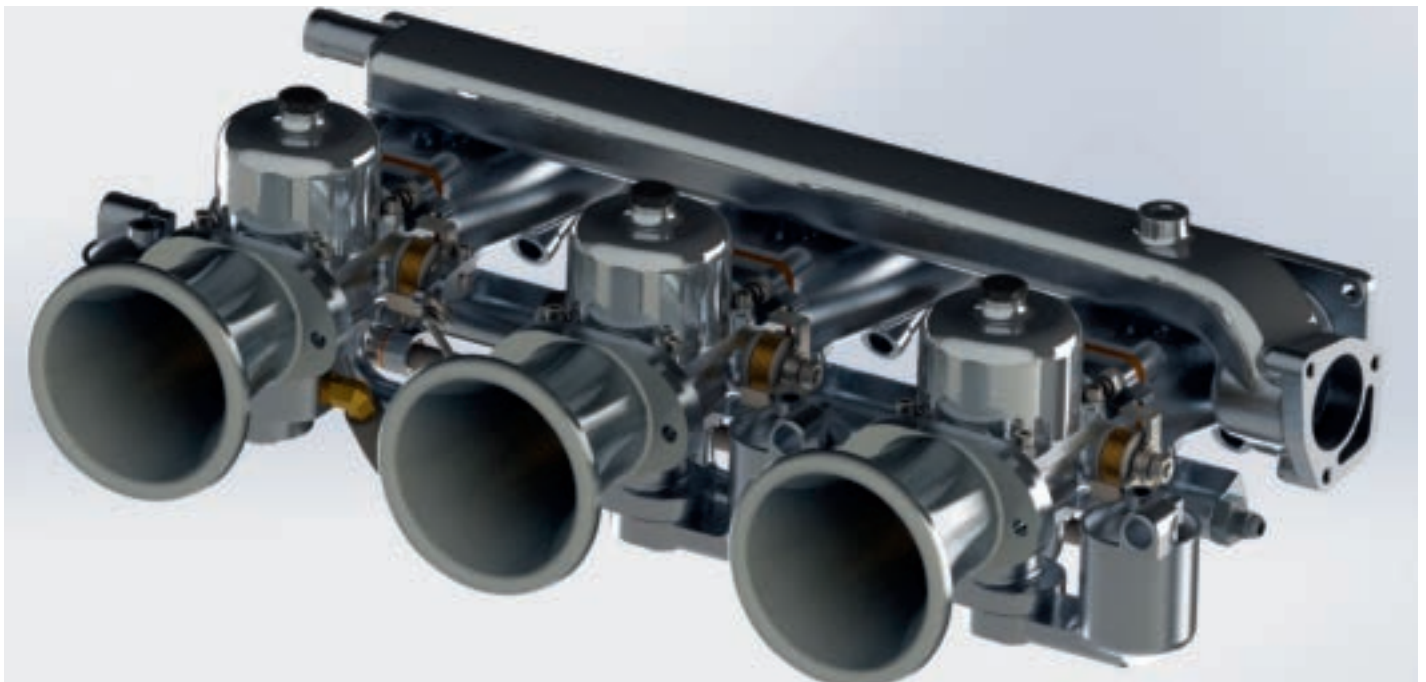
Rendering of SU-lookalike fuel injection that was on show at the Mahwah AGM last March.
