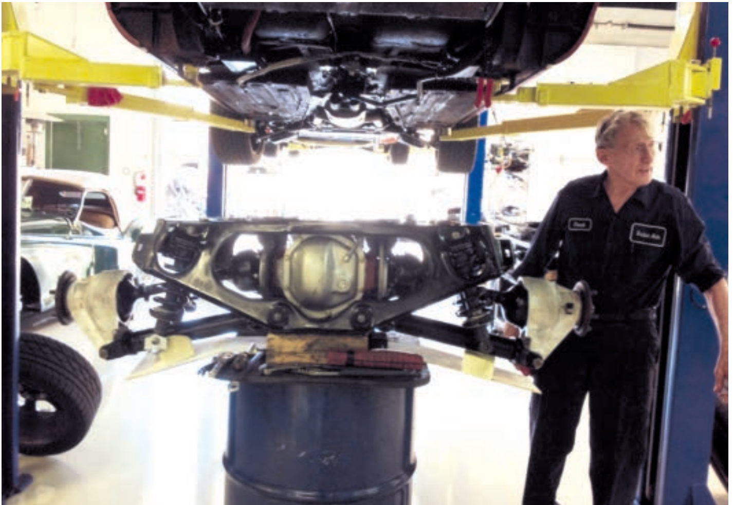
Chuck Banning drops the rear suspension: easy on a rust-free car.
