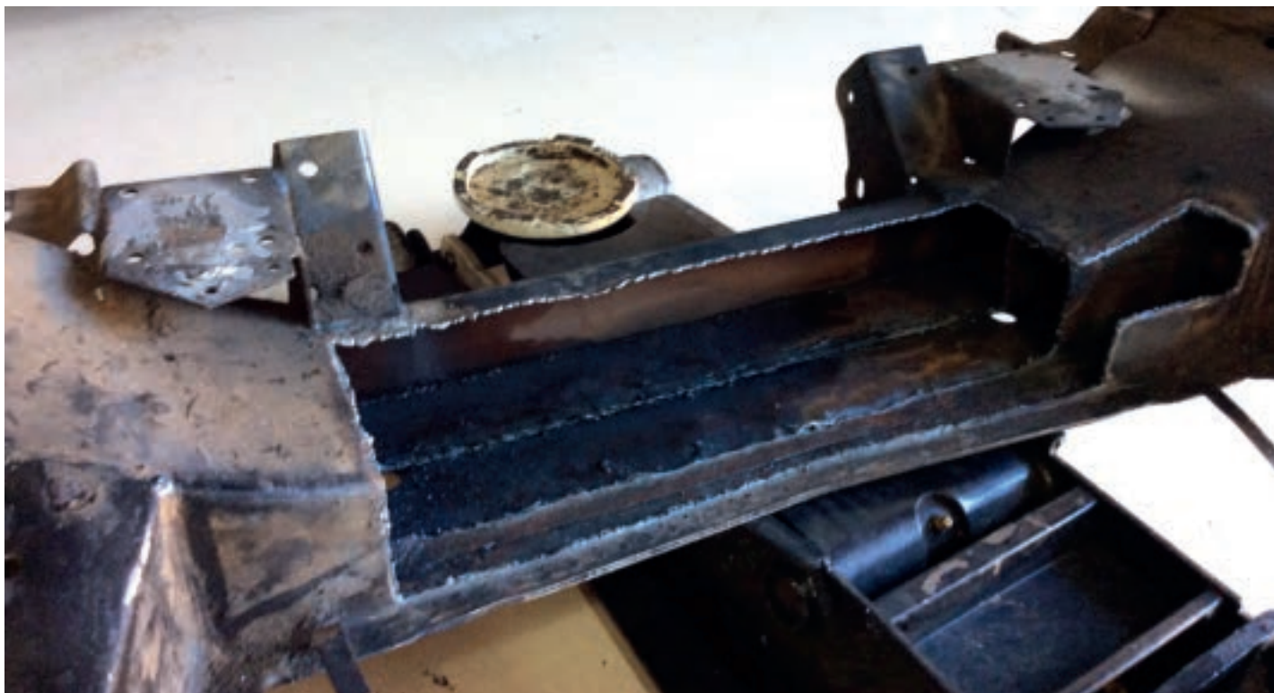
Cutting/resection and rebuilding of the subframe took several trial fits.
