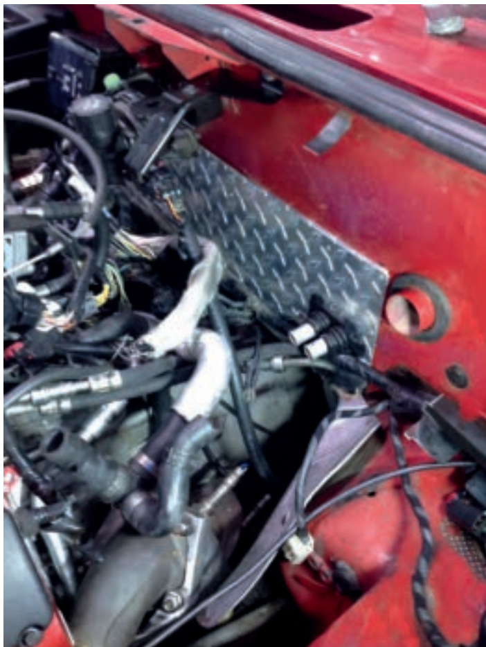
The left front bulkhead rebuilt with diamond pattern alloy plate. Some would choose steel.
