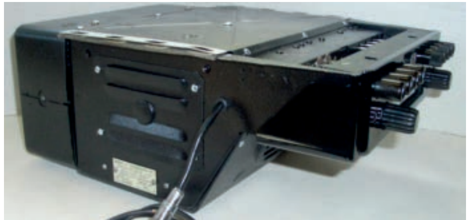
The typical single-unit construction of the 100 series, but the amplifier at the back could be detached if required.
