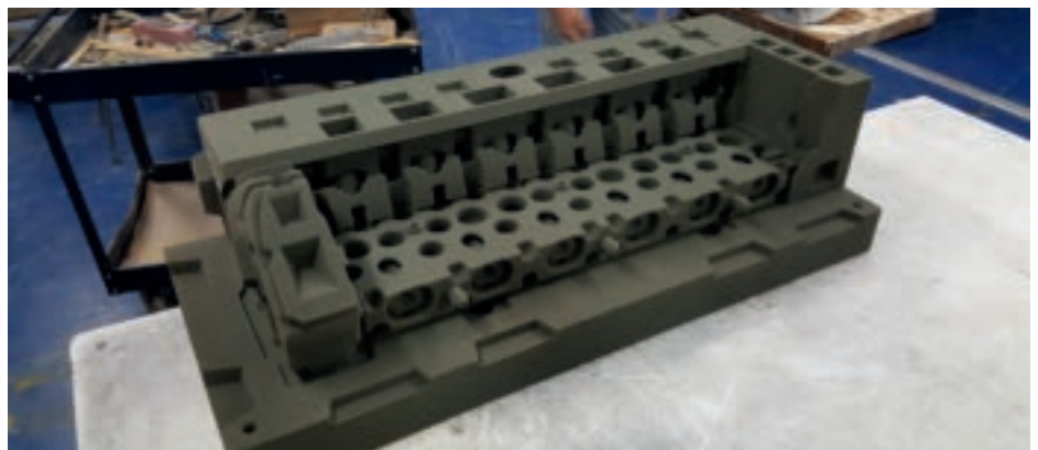
A 3D-printed mold, straight from the CAD program to the finished shape with no human tool or pattern maker involved.
