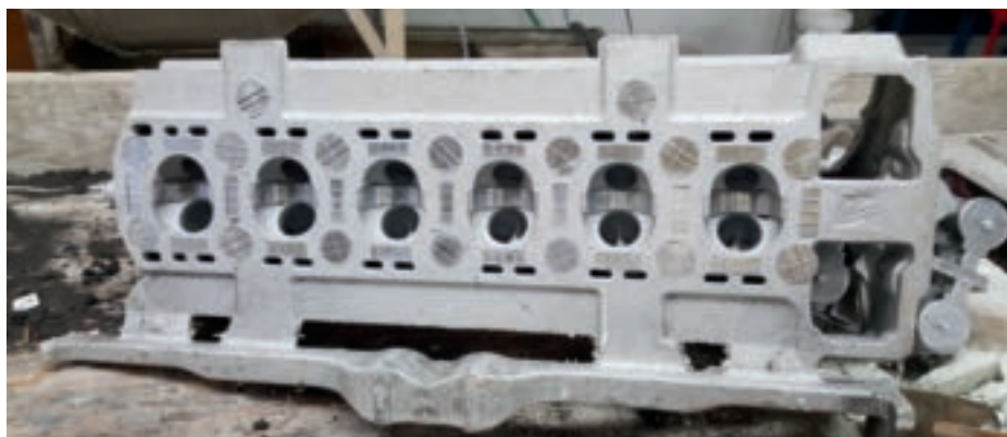
Raw casting, showing the solidified molten metal in the parallel feed channel or 'runner' which fills the mold. The passages to the mold from the runner are called 'sprues' and are usually cut or snapped off as one of the early clean-up stages when cast parts are pulled from the mold.
