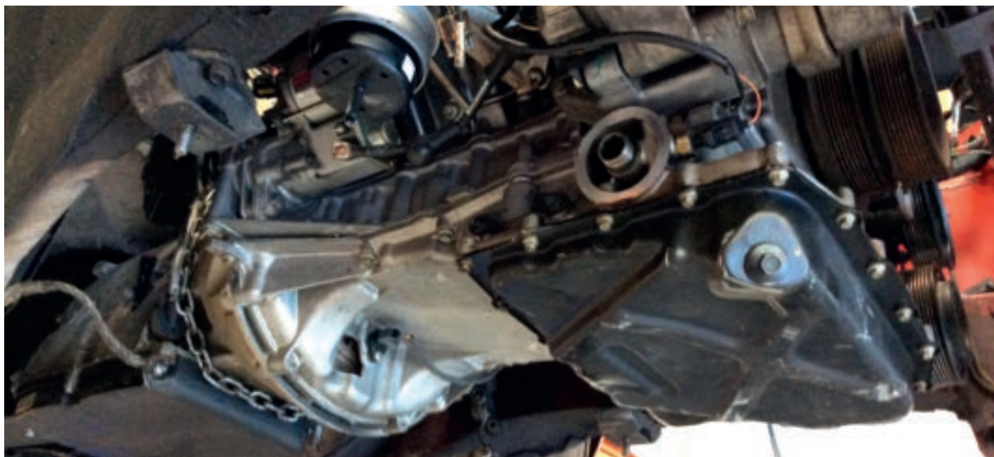
The engine and trans are supported from above whilst checking for fit and position.
