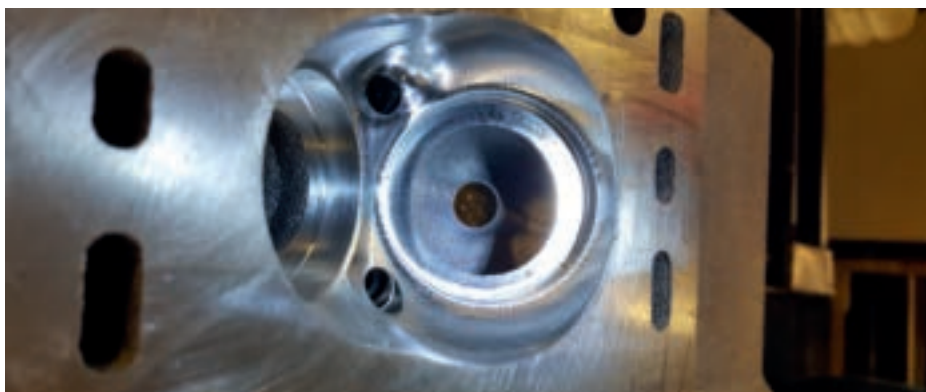
Twin plugs help but are optional. No valve seats fitted yet.
