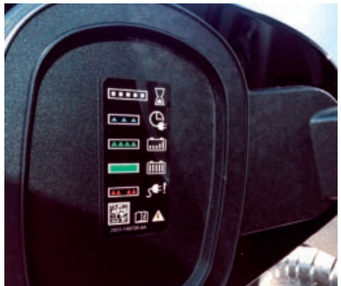
The 'fuel filler' has a legend to decode the five different patterns of battery and charging status.
