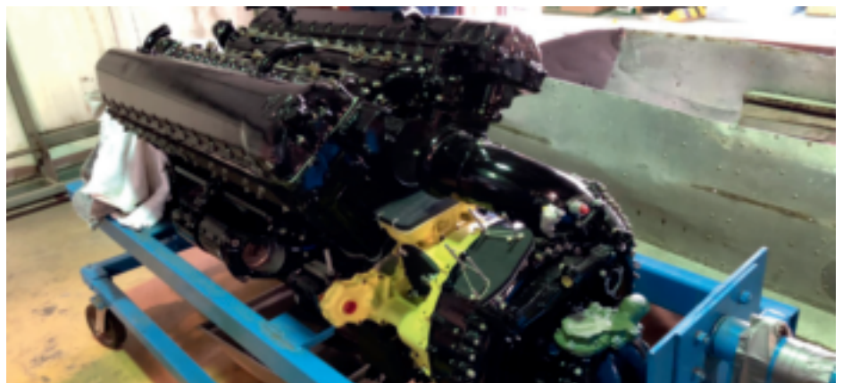
A bigger than average engine stand for each of the Lancaster's four Merlins.
