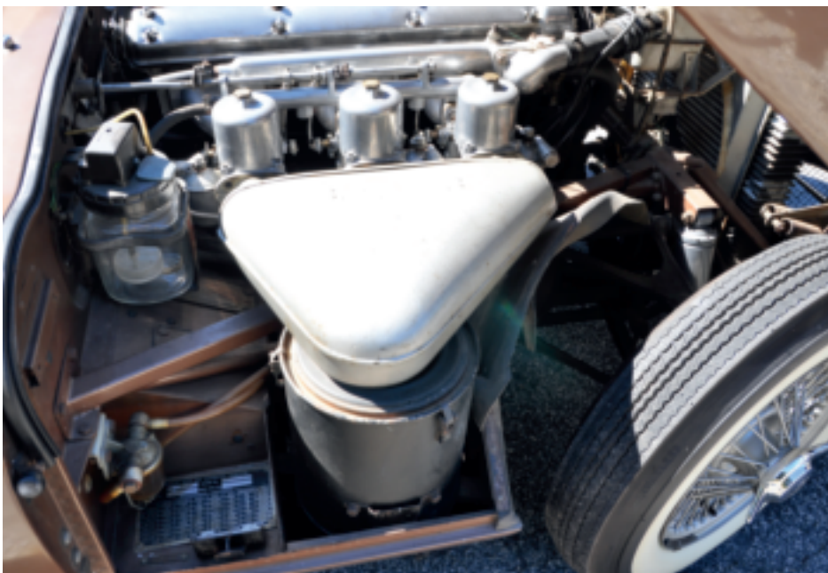
Early carb top linkage, plenum, bonnet catch and reproduction tires.
