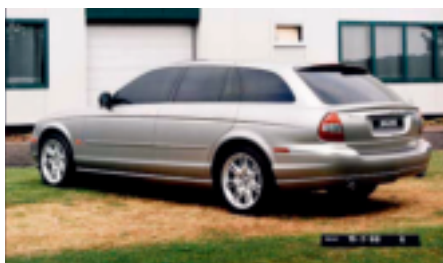
A sports estate version of the S-Type was developed in 1999, with the code initials ALV. Seen here as a double-sided clay model, the proposal was dropped in favour of the X-Type Estate.
