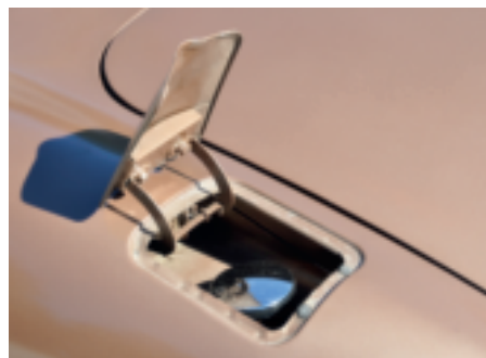
Early filler cap and rectangular filler flap, not tapered.
