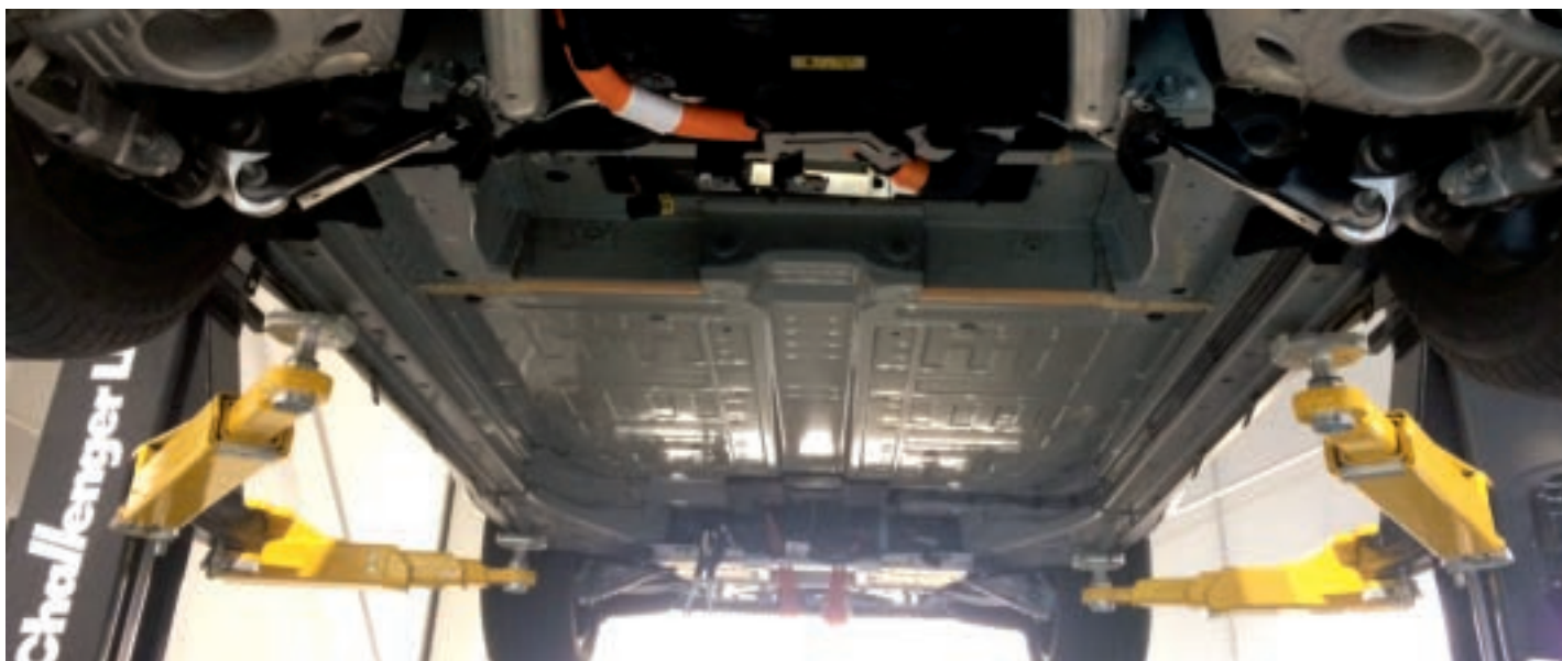
For service, the entire pack is removed from under the car floor. This could perhaps evolve into a possible 'instant refuel' option.
