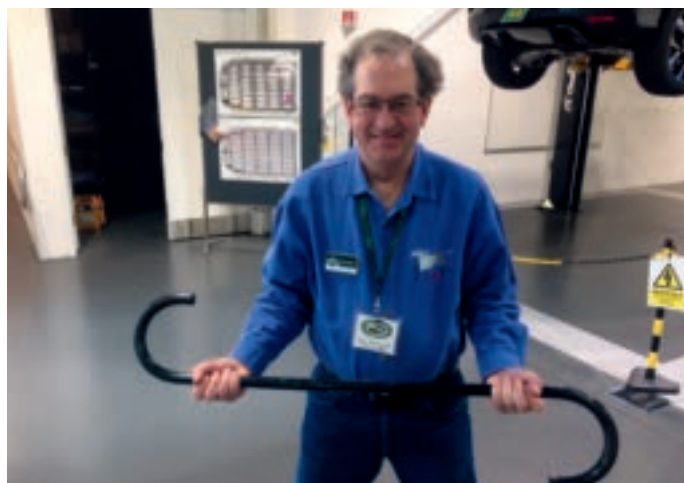
Bob Matejek poses with the deadly-serious carbon fiber rescue hook used to pull injured persons off any power source.
