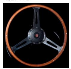
Moto-Lita still manufactures the Derrington wheel today and adheres to the original design although with nine-bolt center mounting.
