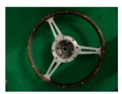
Original Derrington 16" wheel with eight screw mounting and 12 rivets.
