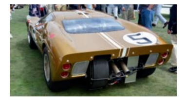
(Left) The intriguing placement of the spare wheel can be seen clearly for this GT40 Mark IIB coupe. One wonders how long it lasted this close to the exhaust? This GT40 was one of only two known examples of the Mark IIB and raced twice at Le Mans.
