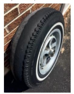
Astonishingly air-tight, despite no tread and riding on the steel belt.
