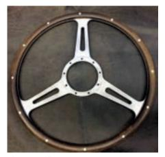
A 1960s 16" Derrington wheel made by Moto-Lita for the Moto-Lita style hub with nine screws.
