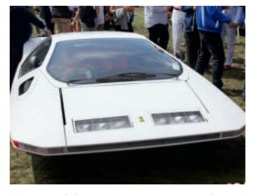
This auto is, believe it or not, a 1970 Ferrari. This 512S Modulo Concept by Pininfarina was unveiled at the 1970 Geneva motor show as a five-liter V12, mid-engined design based on Ferrari's 512S racing chassis. To enter the cabin, the canopy and front of the body slide forward.
