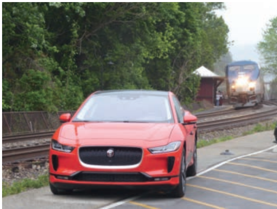
Both vehicles use electric traction motors. One is zero-emissions, one a diesel hybrid.
