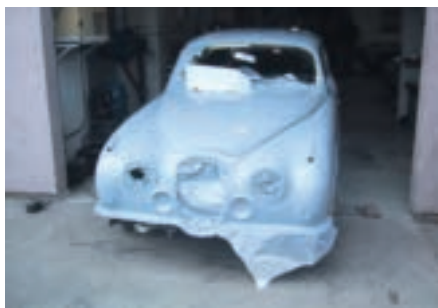
The easy part – putting on a good etch primer. Next came a color 'discussion'.
