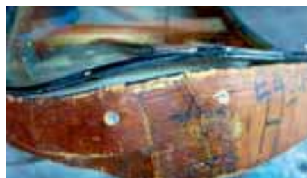
An original 1966 windscreen laid on the original wooden pattern shows the incorrect curvature.
