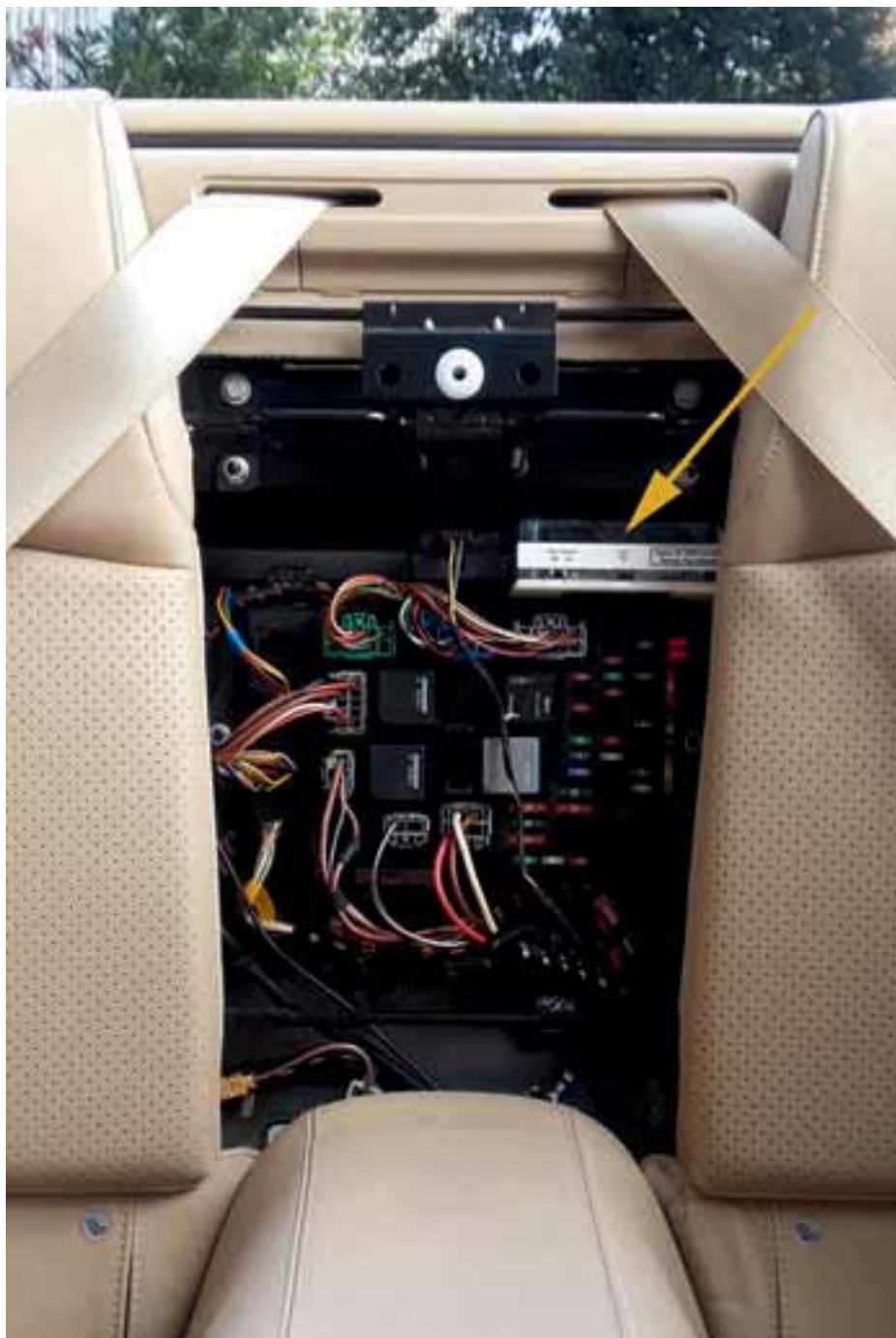
Finished installation with rear center seat back removed to show final placement of the Remote Top Module.
