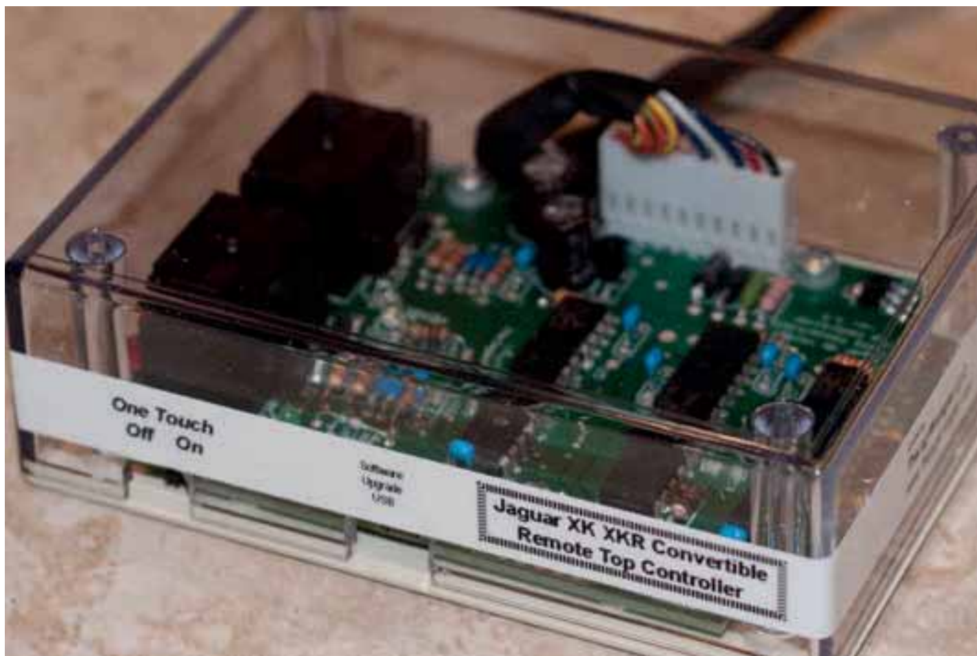
The X150 Remote Top Module – a significant bit of hardware and software engineering.
