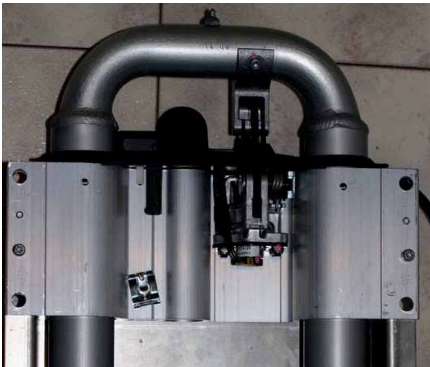
Rollover Protection Device that needs to be removed temporarily from the vehicle for access to wiring at the Roof Control Module.
