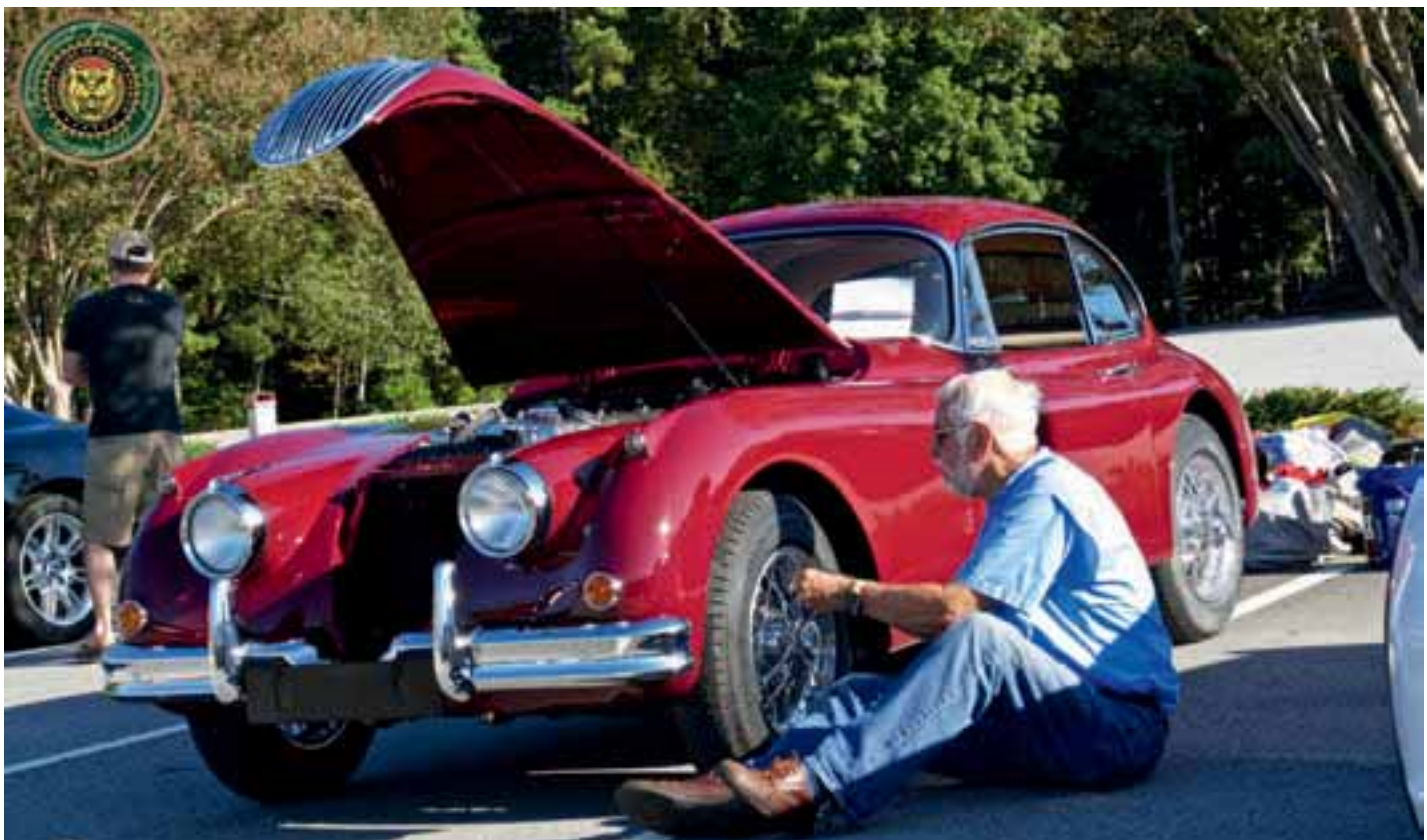
Tom adjusts tire pressures to cut understeer.
