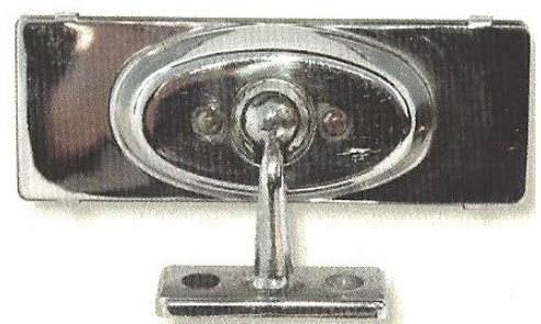
February 1953 onwards, (C.5500) wide flat glass interior mirror, short stem.
