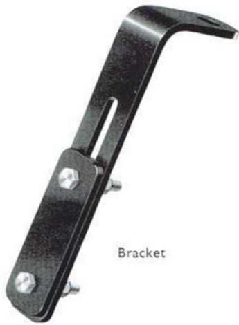
The (056117) universal two-piece, adjustable fog lamp mounting bracket shown above, is NOT an authentic Jaguar factory supplied XK 120 C.2985/86 fog lamp mounting bracket. Therefore, it is 'NON-AUTHENTIC' for judging purposes. Photos provided by Roger Payne.
