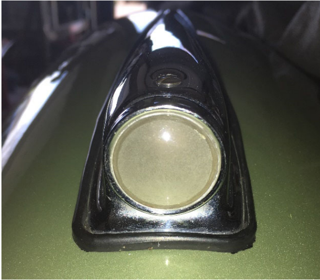
'Original' LUCAS MODEL 490 side lamp with plain, slightly convex, opaque/white lens.
