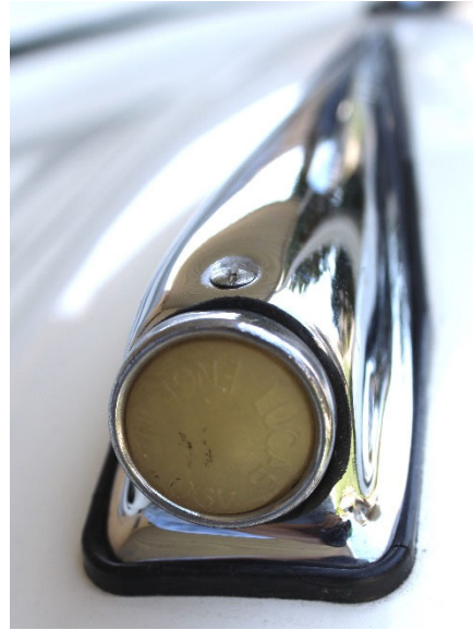
'Original' LUCAS MODEL 490 side lamp NOTE: over time, the lens can turn a 'yellowish' color which is acceptable.
