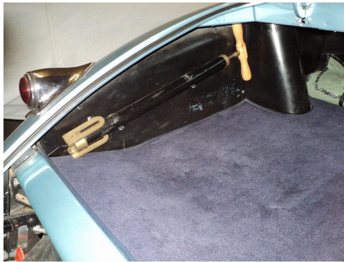
Alloy cars and early steel-bodied cars, until end of 1950, had the tyre pump on left-hand side as pictured above. Alloy cars and early steel-bodied cars, until end of 1950, had the tyre pump clipped onto the left-hand side panel as pictured above. (NOTE, pictured tyre pump with brass feet is a reproduction)
