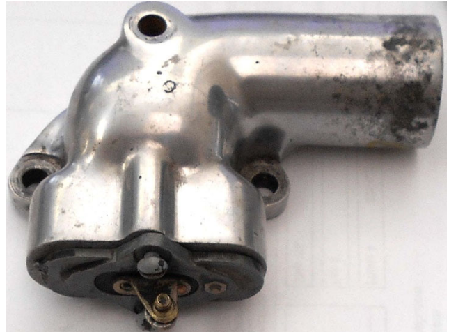
Side view of early water outlet elbow with thermostat switch.
