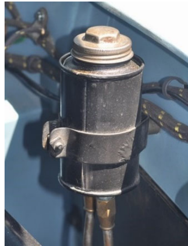
Brake supply tank including cadmium-plated filler cap.
