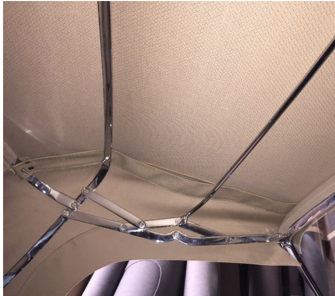
BD.4727 style-2 hoodsticks are chrome-plated and are used with early steel bodied OTS cars until mid-1951.
