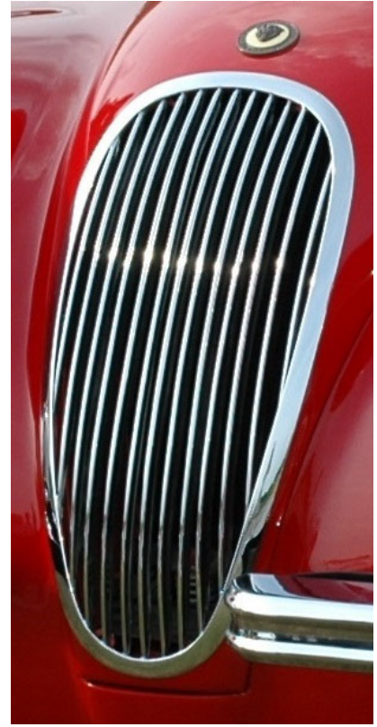
Later grille vanes have rounded leading edges.
