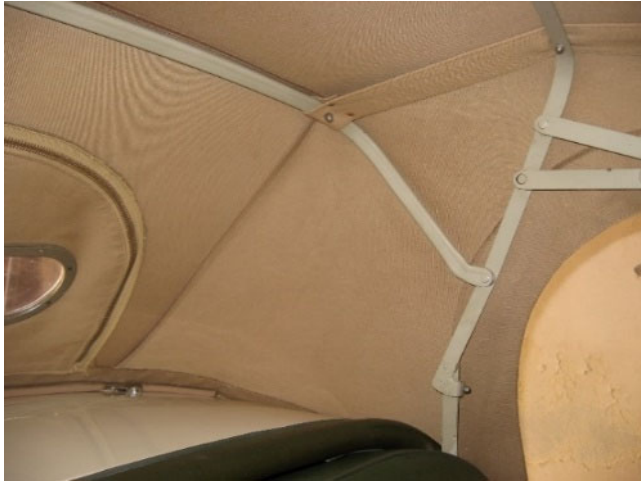
BD.5848 Style-3 hoodsticks are used with the longer hood on later steel-bodied OTS cars.
