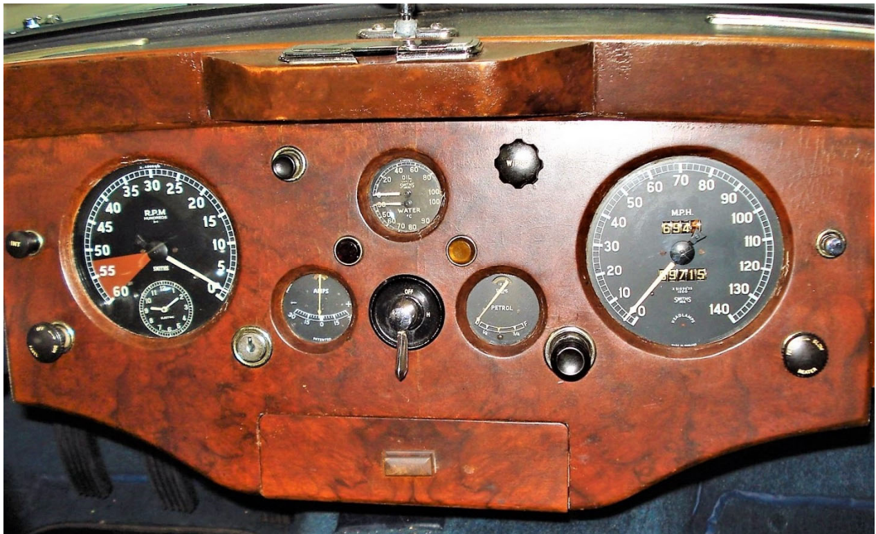
Instrument Panel Assembly from a June 1953 DHC, typical of all 'Later FHC/DHC' XK120 (photo supplied by Cliff Lewis) — see text and NOTES below regarding detail of the gauges, switches and warning lights, and any variations.
