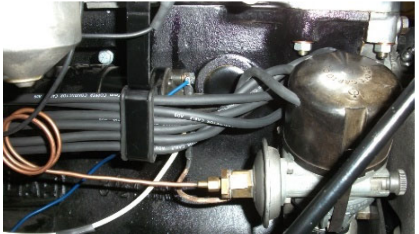
After exiting the horizontal Distributor Cover, the High-Tension Leads are grouped through a flat and horizontal clip with a rubber grommet. A copper Vacuum Advance Tube is connected to the vacuum-advance unit of the distributor. (NOTE: The white lettering on the high-tension leads, is NON-AUTHENTIC. The flat clip should be horizontally oriented, not vertical as shown. (NEED A BETTER PICTURE) ).
