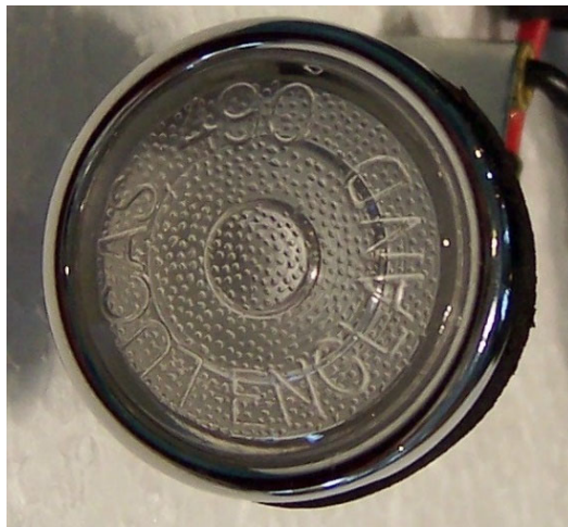
'Replacement' side lamp lens, marked 'LUCAS 490 ENGLAND' with basic bullseye/ring pattern.
