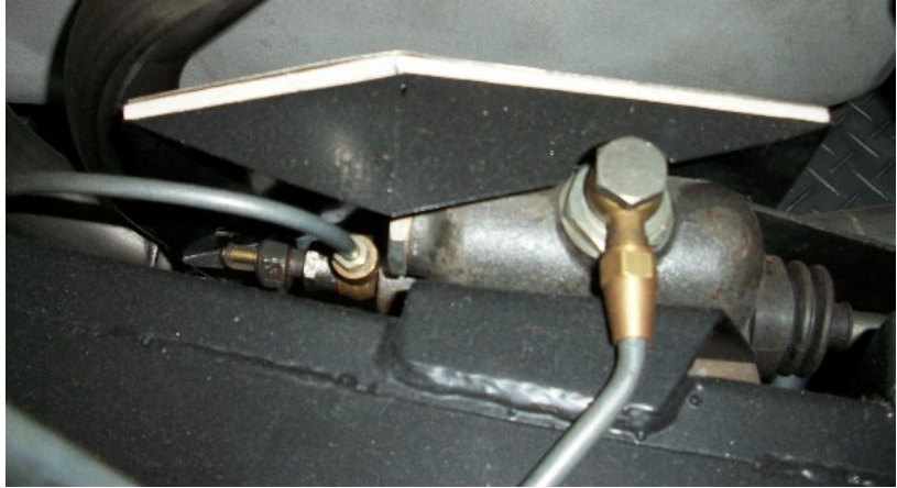
Brake master cylinder assembly, stop light switch fitted to the front, heat shield and supply line coming from the supply tank assembly above.
