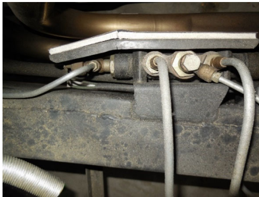
Photo of an incorrect LHD Dual Master Cylinder arrangement, with the Light Switch mounted at the front (as is the case for RHD), and not correctly on top as shown in adjacent photo.
