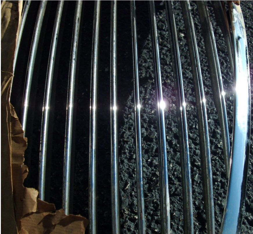
Early cars (up to about 1951) have grille vanes with raised-flutes on leading edges.
