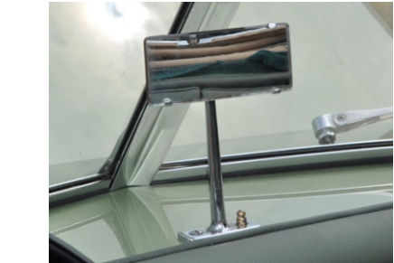
From August 1950 to February 1953, (C.4097) narrow convex glass interior mirror, long stem.
