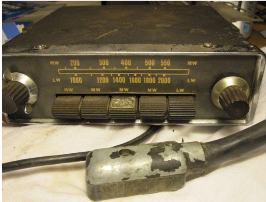
Early C.4063 car radio assembly Radiomobile model RP.100, with "His Master's Voice" on the middle button.
