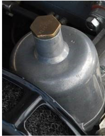
From May/June 1950 onwards H6 carburetors now have a 'short neck' suction-chambers, initially without any side rib as shown. (NOTE: hexagon oil-caps should be dull-nickel plated)
