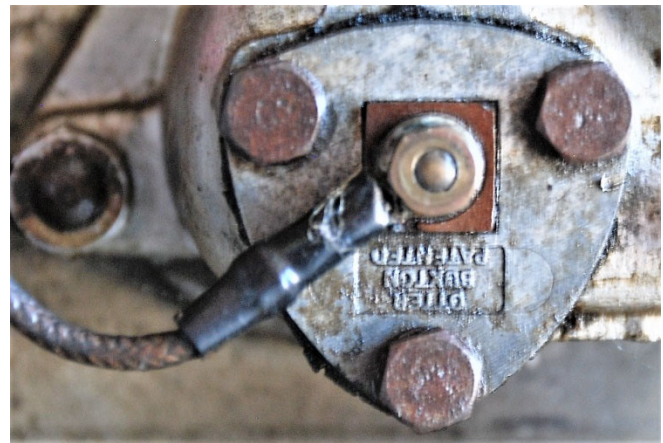
1950/51 onwards, second variant C2474 Otter Switch (cable to the starting-carburettor is connected)
