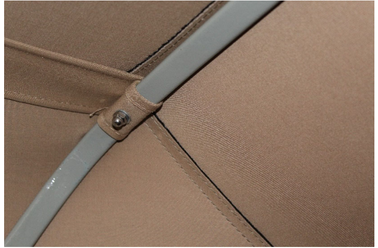
BD.5848 Style-3 hoodsticks are used with the longer hood on later steel-bodied OTS cars.
