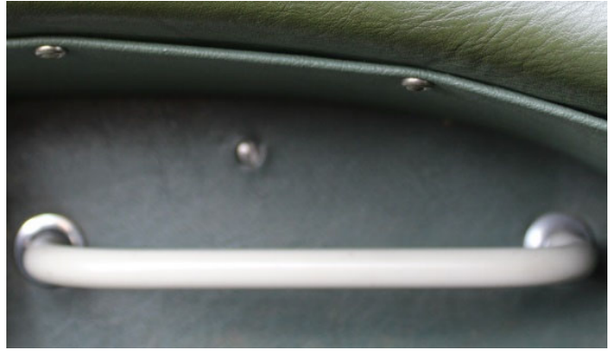
Later steel-bodied cars grab rail bar painted greenish/grey. Photo © Copyright 2002 by Urs Schmid.
