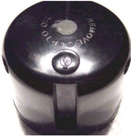
Early Distributor Cover up to February 1953, with horizontal High-Tension Lead outlets.
