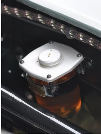
Brake fluid supply tank assembly, showing the glass body and filler cap.
