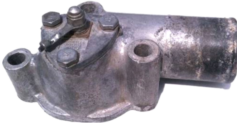
Underside view of later Water Outlet Elbow and second variant C.2474 Thermostat (Otter) Switch, with electrical connection.
