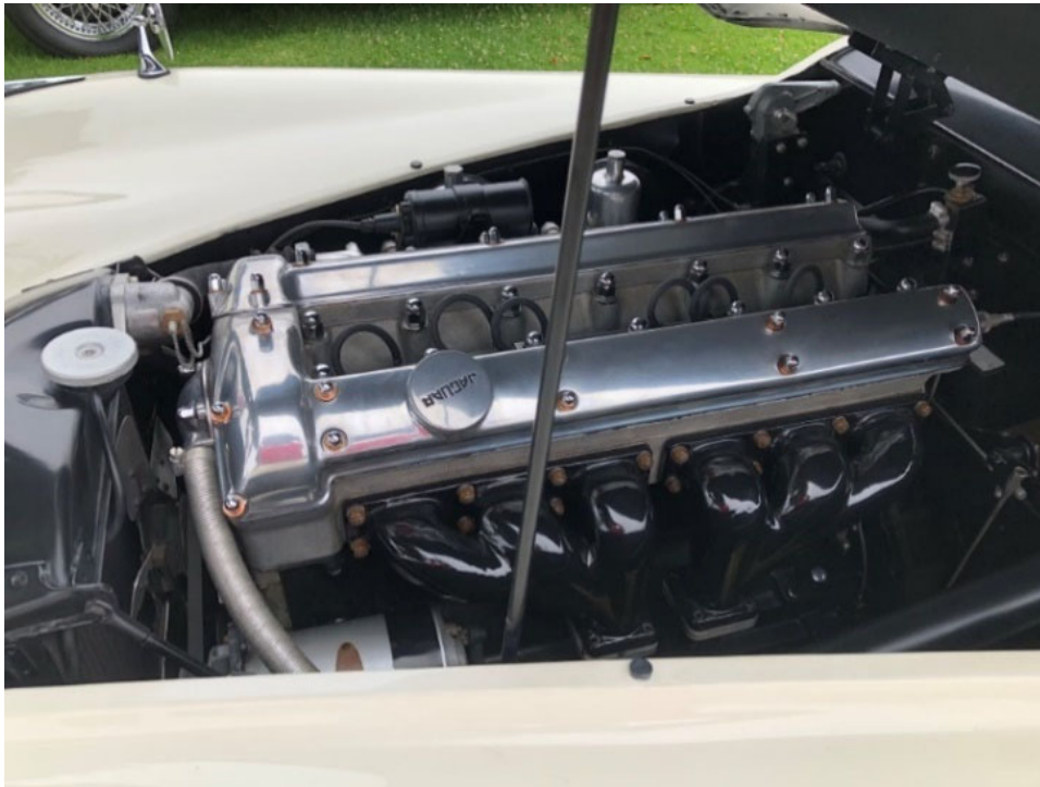
Early Steel-Body Cylinder Head. NOTE: Ignition wires come up from the back of the head. (Photo by Robert Sheridan)
