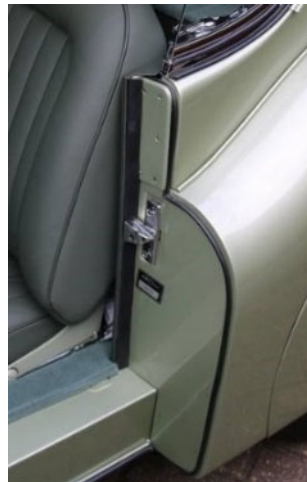
NOTE: FHC/DHC un-painted chrome dovetail strikers are NON-AUTHENTIC.
