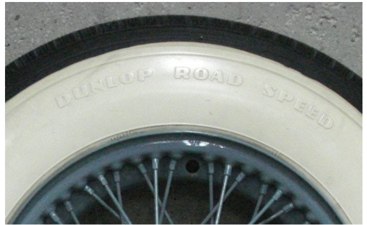
An original June 1953 DUNLOP ROADSPEED Tyre with WHITE sidewalls as available as an OPTIONAL-EXTRA for XK 120 from May 1953 onwards. (Photo by Cliff Lewis)
