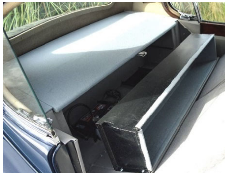
View of parcel box open. The parcel box swings forward on two hinges, exposing the batteries.
