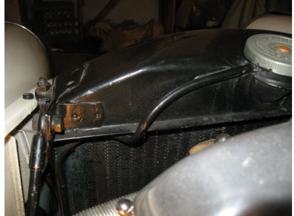
View of radiator overflow tubing correctly routed. Any other routing is NON-AUTHENTIC.
