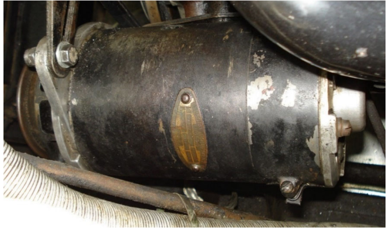
1953 generator body and cover-band painted black. (Photo by Cliff Lewis)
