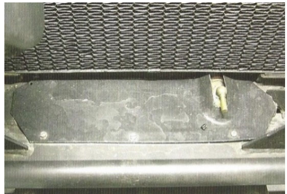
Radiator drain and lower air deflector. NOTE: The tie-rod is always painted semi-gloss black. (Photo © Copyright 2002 by Urs Schmid)
