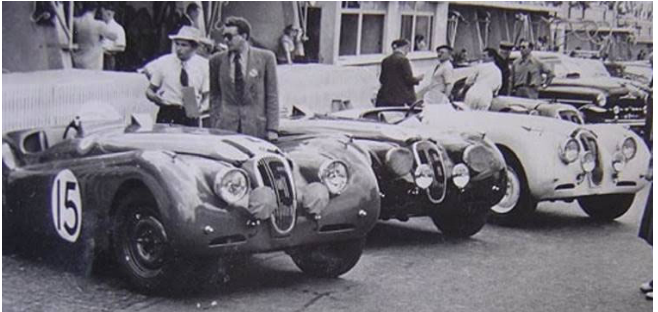
The three 'works team' XK120's (June 1950) Le Mans 24-hour race, showing their factory fitted fog lamps, mounting brackets and black plastic sleeve covered wiring cables routed through the front wings. Photo provided by JDHT.
