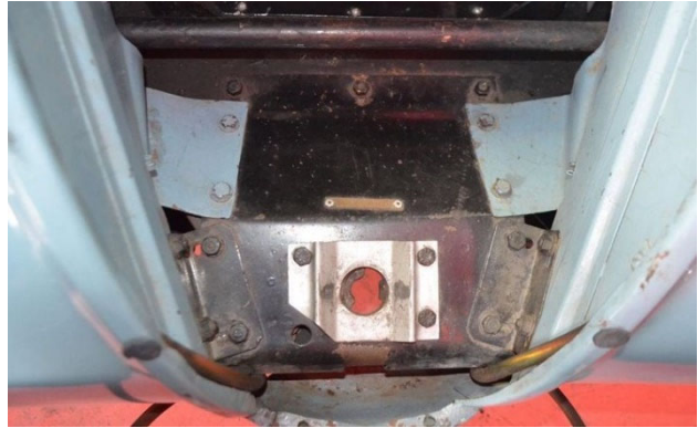
Later steel-bodied cars were painted at Brown's Lane paint shop. NOTE: the two plastic tubes at forward-corners of mounting-plate are non-original. (Photo of 1954 DHC by Steve Kennedy)
