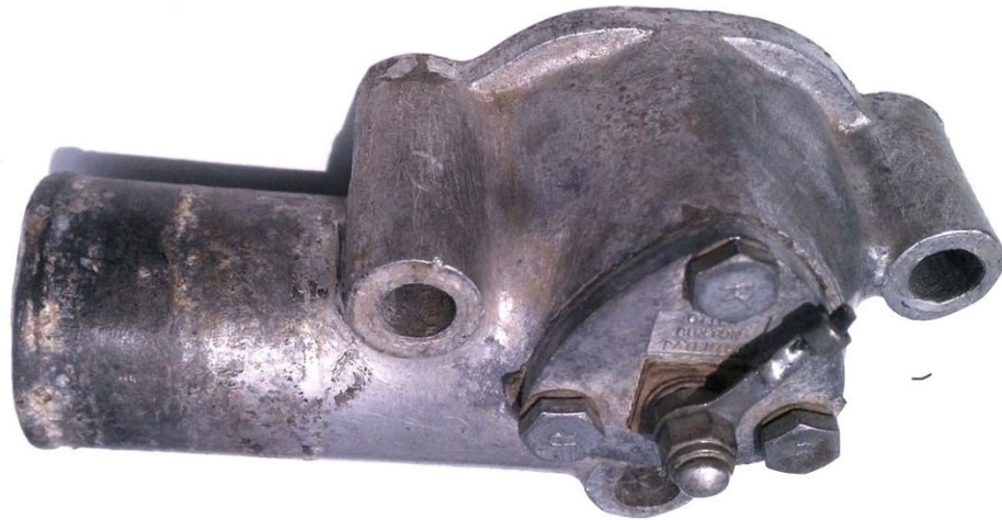
View of later Water Outlet Elbow and second variant C.2474 Thermostat (Otter) Switch, with electrical connection. Note: when the Water Outlet Elbow is correctly installed, the lettering is upside down).
