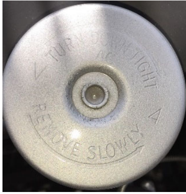
Original cadmium-plated XK120 radiator-cap, AC (UK) 'circular' model RB4, stamped '4' denoting 4 psi.
