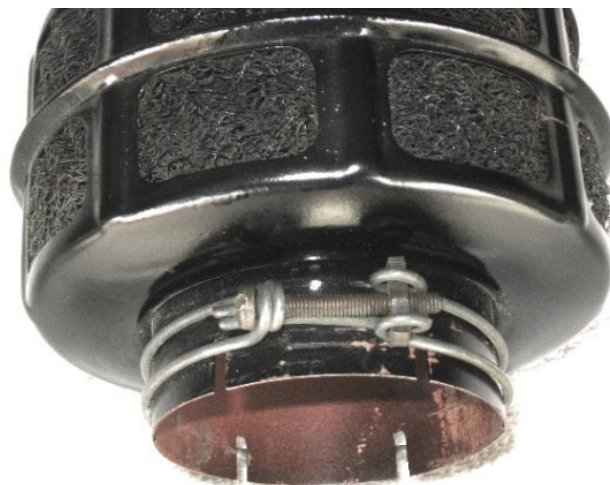
FHC/DHC air cleaner, view of large wire clamp on left-side.
