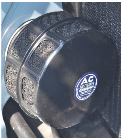
FHC/DHC air cleaner exits from right-side wing.
