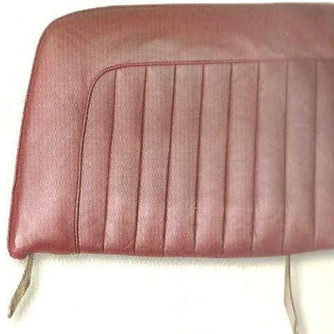
Later FHC flat seat backs/squabs with 9 flutes. (Photo © Copyright 2002 by Urs Schmid)
