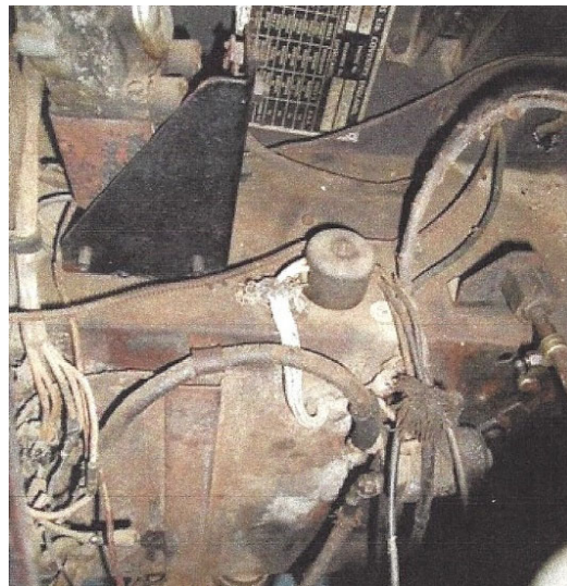
C.5258 junction box for C.5260 engine harness. FHC 679240 (January 1952).
