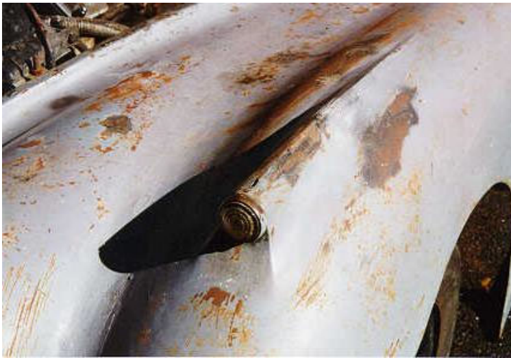
FHC chassis no. 679012 Mark V sidelamp housing. Observed BEFORE restoration. (Photo by Carl Hanson, owner)
