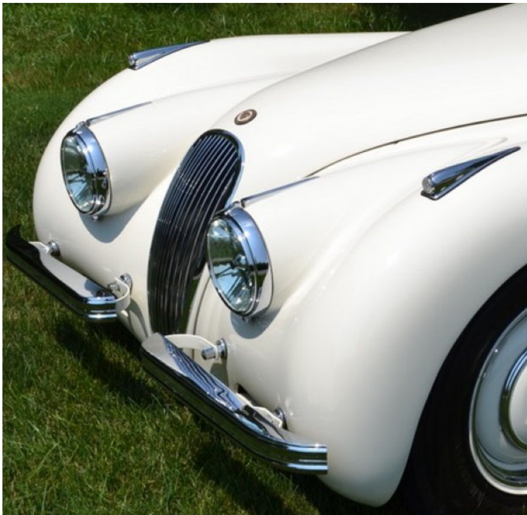
Notice that early Jaguar XK 120 cars Spring Bar assemblies were painted body color. (1949 to December 1952)
