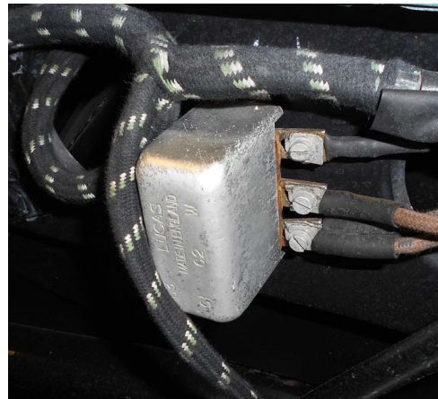
Early steel-bodied car horn relay, dull-cad finish.
