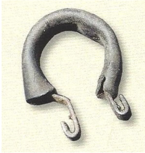
Metal retainer clip used to support wiring harness. (Photo © Copyright 2002 by Urs Schmid)
