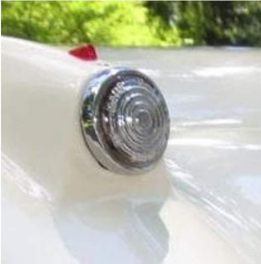
From chassis no 672927 onwards, side lamps with turn signal, used Lucas Model 513 lens with LUCAS and 513 lettering molded in..
