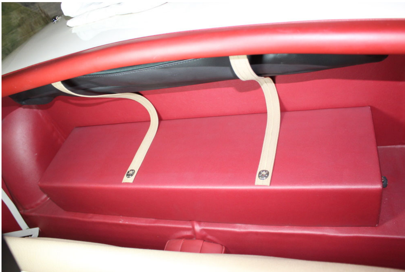
OTS Battery Cover is secured by two Dzuz fasteners, pictured below. Notice the two canvas straps used to secure the style-2 backlight when it is folded down. Style-2 Hood Cloth Assembly was used from Feb 1951 to Jan 1953). (Photo by Robert Sheridan)
