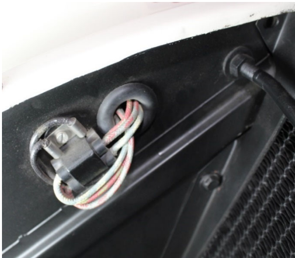
5-Way Rubber Connector, right-side, in front of the Radiator. (Photo by Robert Sheridan)
