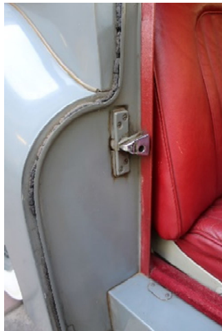
Original, unmolested 1954 DHC dovetail striker screw faces are painted body color.
