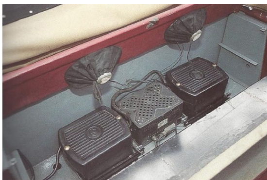
FHC/DHC Speakers under the Parcel Shelf and Power Amplifier between Batteries. (Photo © copyright 2002 by Urs Schmid)
