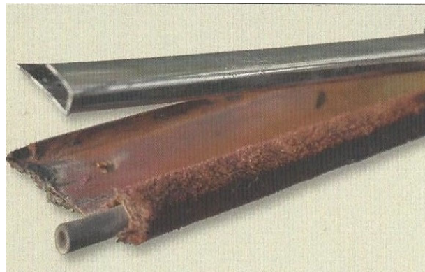
Steel-bodied carpet with chrome carpet rail and draft excluder (Furflex) along the door sill and up each 'A and B' door post. Photo on left by Robert Sheridan. Photo on right © Copyright 2002 by Urs Schmid.
