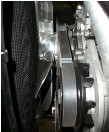
A 5-blade cast-aluminum fan, is used until May-June 1952. (Photo by Robert Sheridan)
