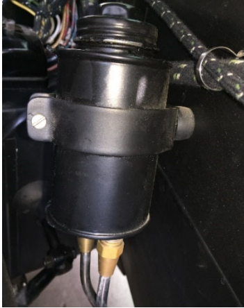
Brake supply tank including black painted filler cap. Photo by Dick Cavicke.
