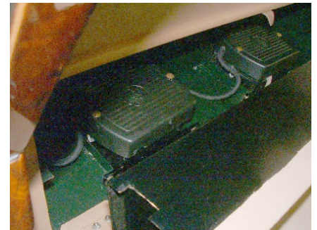
Both DHC and FHC have Two 6-volt Lucas battery's, and three battery cables like OTS.
