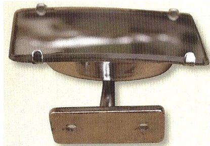
From March 1950 to August 1950, (C.2887) narrow convex glass interior mirror, short stem.
