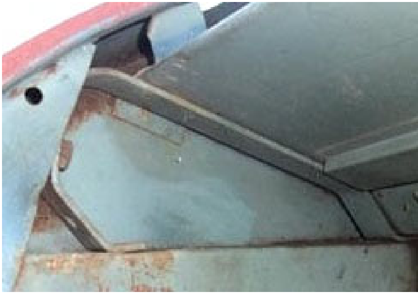
Over-rider brackets are used to mount the rear over-riders (bumpers)
