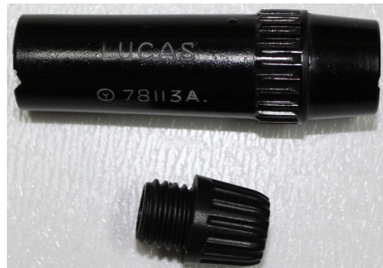
Six Sparkplug Suppressors are used when XK120s are fitted with a Radiomobile or Emitron Radio. (Photo by Robert Sheridan)
