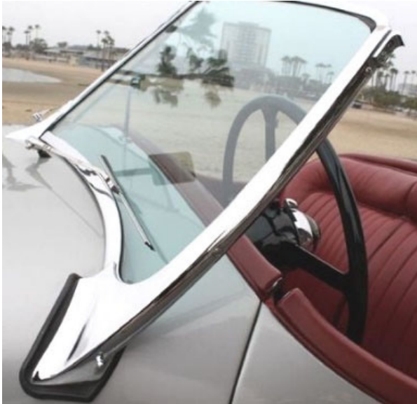
OTS side post with hood clamp, 'Lift-the-Dot' stud and rubber mount. Note the excessive gap in the crash roll.
