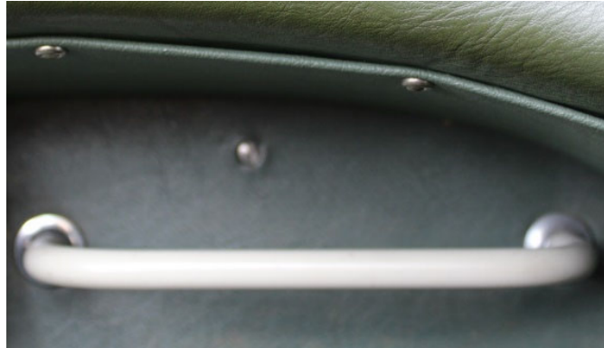
Some early steel-bodied cars grab rail bars are painted greenish/grey. (Photo © copyright 2002 by Urs Schmid)
