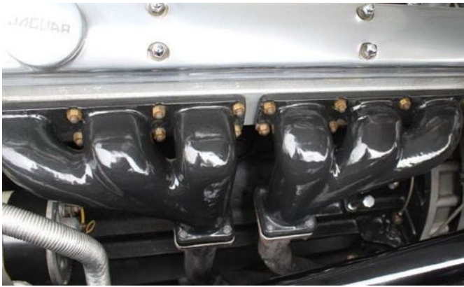
Porcelain coated exhaust manifolds are fastened by bronze nuts on single coil spring washers. (Photo by Robert Sheridan)
