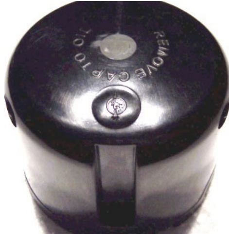
Early Distributor Cover, up to Feb 1953, with horizontal high-tension lead outlets. (Photo by Robert Sheridan)
