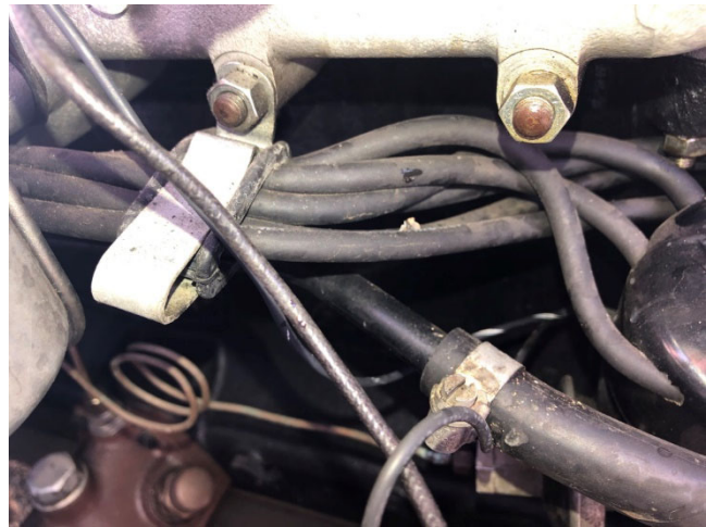
After exiting the horizontal Distributor Cover, the High-Tension Leads are grouped through a flat/vertical clip (with rubber grommet. A copper vacuum tube is connected to the vacuum-advance of the Distributor. NOTE: White lettering on High-Tension Leads, is NON-AUTHENTIC. (Photos by Robert Sheridan)
