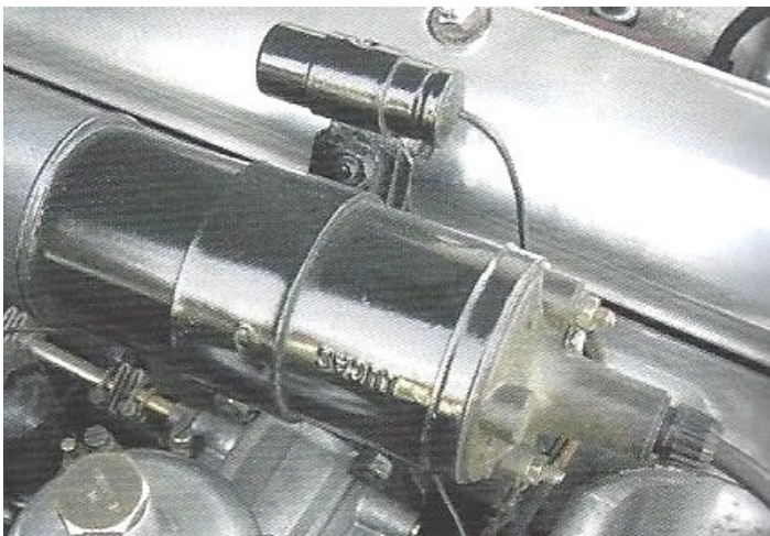
Coil condenser for cars fitted with a radio. (Photo © copyright 2002 by Urs Schmid)
