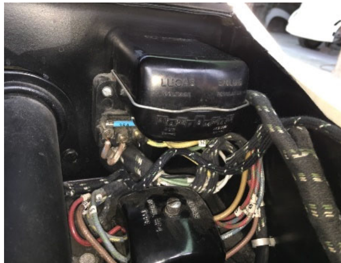
OTS, (C.2530) control box (voltage regulator) and (C.2829) fuse box containing four 35-amp fuses.
