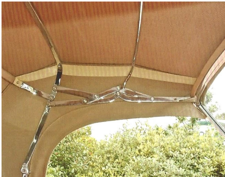
BD.3317 style-1 hoodsticks (metal frame) are chrome-plated and are used with the 'short hood' on the alloy and earliest steel bodied OTS cars.
