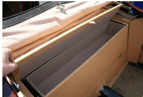
View of the parcel box lid open, same as FHC. Parcel box swings forward on two hinges like FHC.
