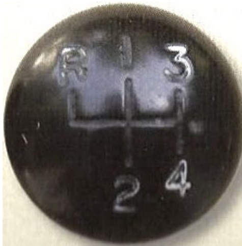
NOTE: Some early alloy body XK 120s have been seen with Gear Shift Knob with a raised shift pattern.
