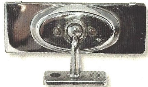
February 1953 onwards, (C.5500) wide flat glass interior mirror, short stem.
