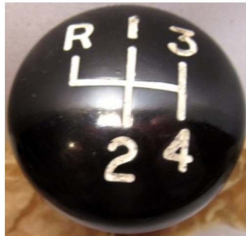
Steel-bodied XK 120s all have a tear-shaped Gear Shift Knob with a flat shift pattern.
