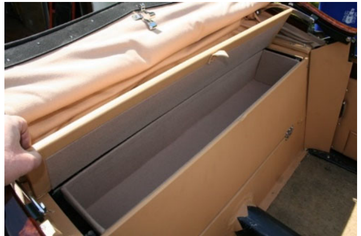
DHC parcel box lid open. The parcel box swings forward on two hinges like the FHC.
