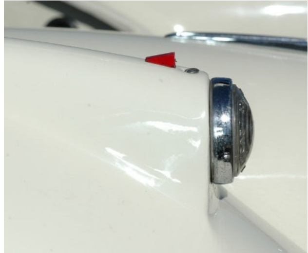
The jewel is positioned correctly and a thin rubber gasket is between the body and side lamp.
