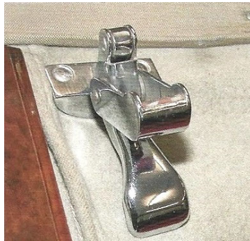
Toggle clamp for securing the hood at left-side and right side.
