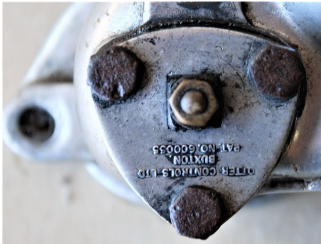
March 1950 onwards, first variant C2474 Otter Switch (cable to the starting-carburettor is removed)
