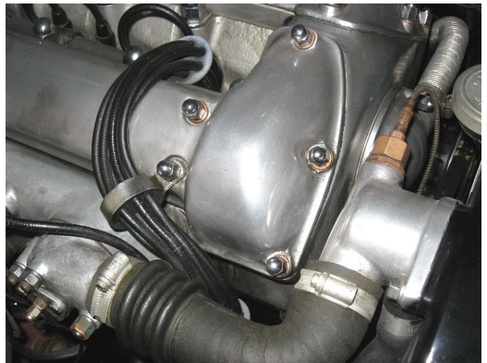
Later Cam cover with 11 studs and dome nuts
