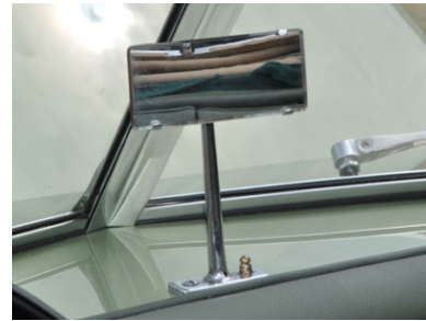
From August 1950 to February 1953, (C.4097) narrow convex glass interior mirror, long stem.
