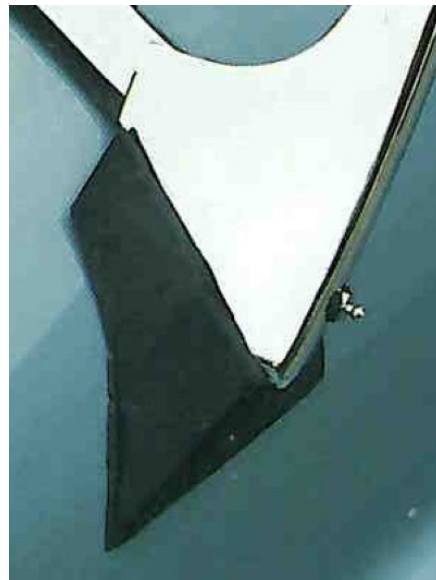
Sample 'Tenax' Stud, used on Alloy and early steel-bodied cars. (Photo @ Copyright 2002 by Urs Schmid)
