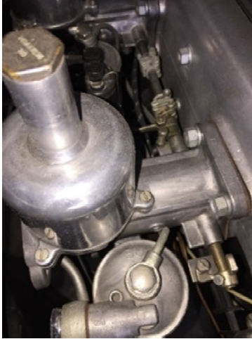
Earlier variant H6-model SU carburetor as used up until May/June 1950, with 'tall-neck' suction-chambers. (NOTE: hexagon oil-caps should be dull-nickel plated)
