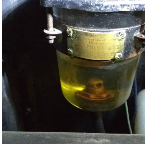
View of FLUID LEVEL tag riveted to the brake fluid ring bracket.
