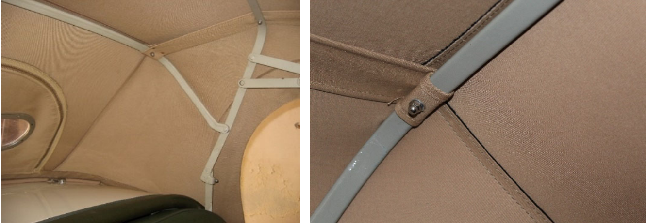
BD.5848 Style-3 hoodsticks (metal frame) are used with the longer hood on later steel-bodied OTS cars.
