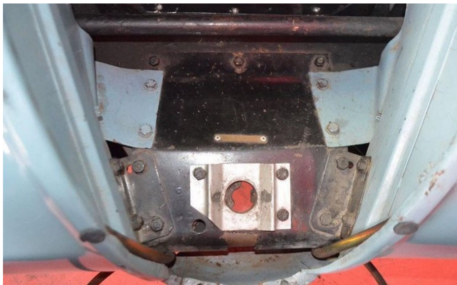
MADE IN ENGLAND tag location. NOTE: the two plastic tubes at forward-corners of mounting-plate are non-original. (Photo of 1954 DHC by Steve Kennedy)
