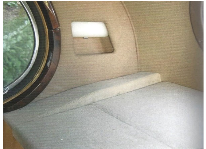
FHC later parcel box covered in Moquette. (Photos on left © Copyright 2002 by Urs Schmid)
