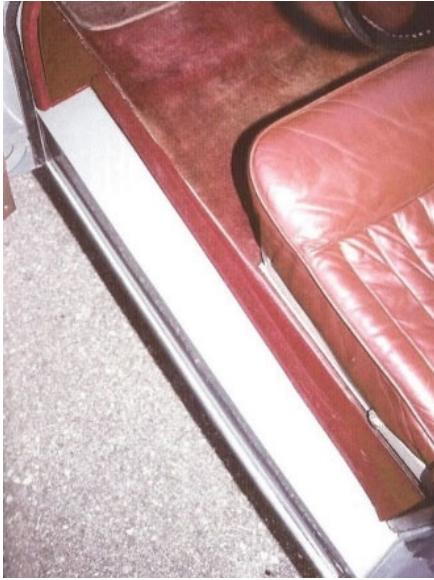
FHC and DHC trim fillet along the door sill, with draft excluder covered in Moquette.
