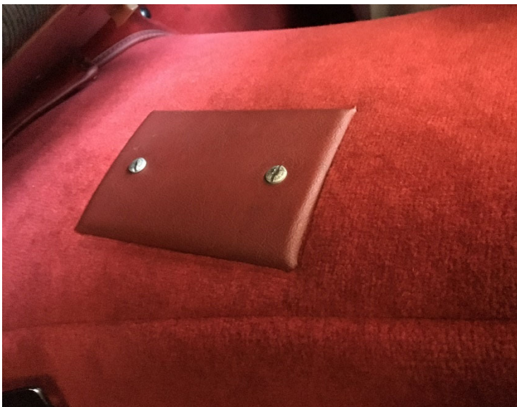
Transmission dipstick cover with 2 Oddie stud fasteners. (Photo on left by Robert Sheridan. Photos on the right © Copyright 2002 by Urs Schmid)
