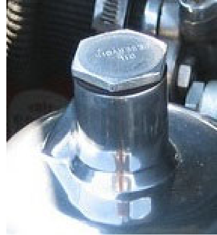
The oil-cap was initially dull-nickel plated, but from 1954 was cadmium-plated, and has stamped in OIL RESERVOIR. The fiber-washer underneath the oil-cap was thin and barely visible, a tan-color initially, but usually black. (NOTE: the rib on the side of neck is an air-vent)
