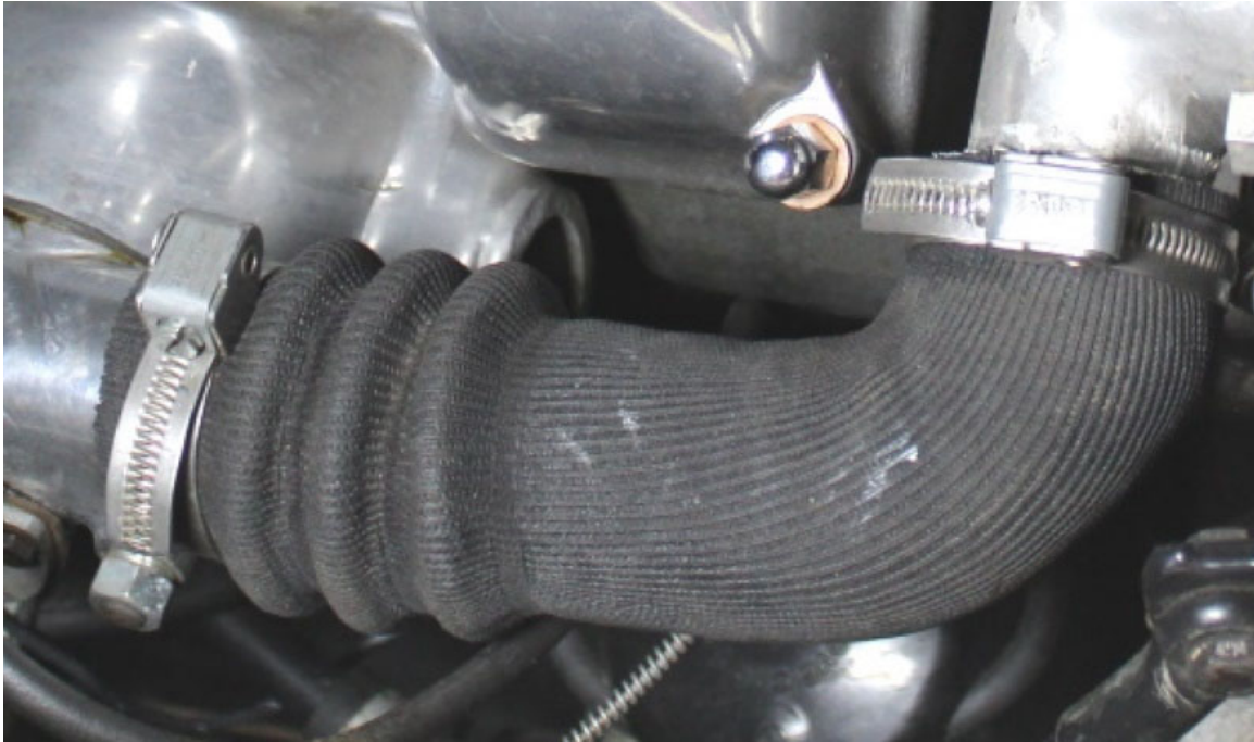
Typical period authentic Top Water Hose, 'Stockinette' covered, and three-ribs. (Photo by Robert Sheridan)
