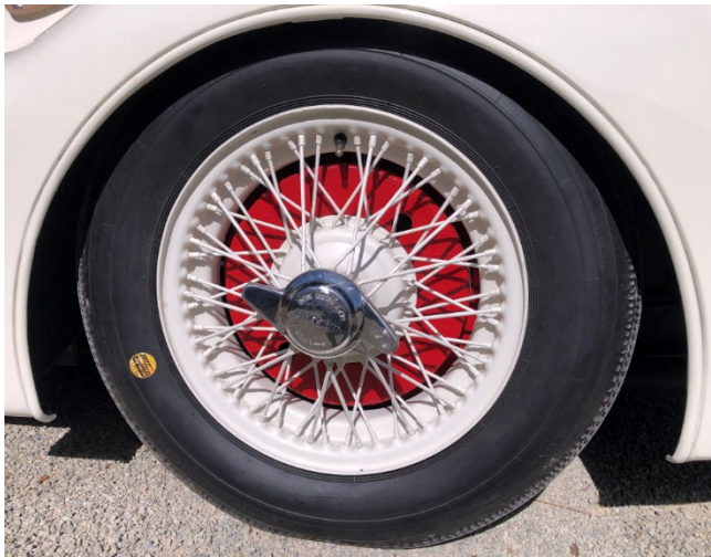
Left: Early XK 120 Painted Wire Spoke Wheel (Photo by Robert Sheridan) Right: Later Steel XK 120 Chrome Wire Spoke Wheel.
