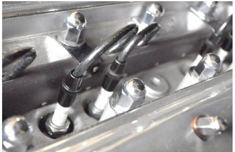
Champion spark plug terminals are fitted to spark plugs from December 1952 onwards. (Photo © Copyright 2002 by Urs Schmid)
