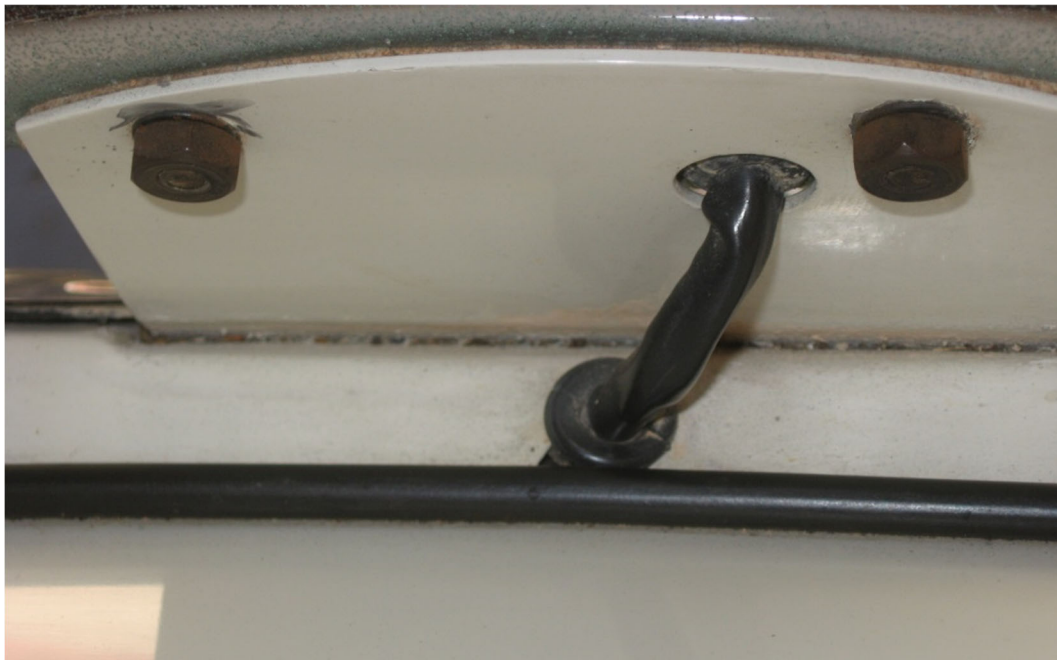
Reverse Lamp Mounting Plate, top-rear view showing black-oxide studs, nuts and black plastic cover surrounding the wiring harness. (Photo by Robert Sheridan)
