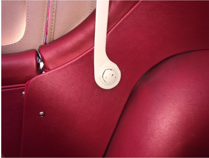
The Hoodsticks (metal frame) Assembly Pivot Screw securing Hoodsticks (metal frame) to left-side/right-side. (Photo by Robert Sheridan).
