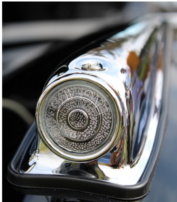
Replacement side lamp lens, marked 'LUCAS 490 ENGLAND' with basic bullseye/ring pattern.
