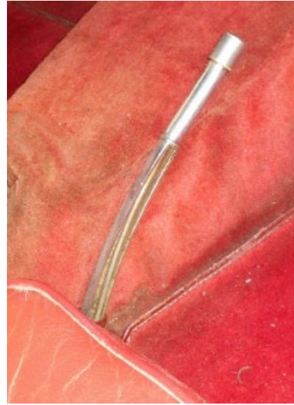
Curved Handbrake from June/July 1954 onwards,
