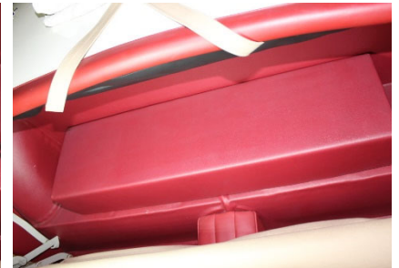
Battery box installed over the batteries.
