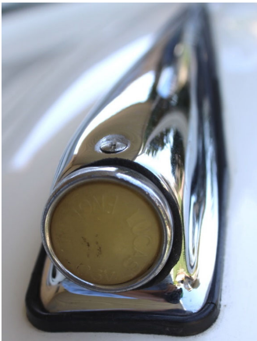
Original LUCAS MODEL 490 side lamp with plain, slightly convex, opaque white or yellow lens. (Photo by Robert Sheridan)
