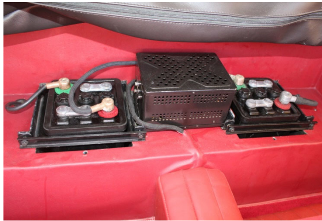
NOTE: Battery cables are covered with braided cloth from the factory.
