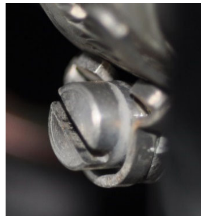
XK 120 style CHENEY Clip, with round Cheese-Head drive-screw
