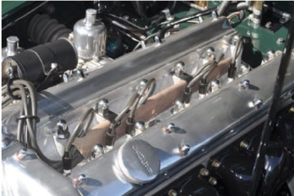
Later Steel-Body Cylinder Head. NOTE: ignition wires come across the front RH cam cover.
