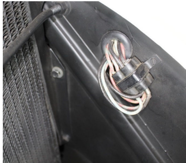
10-Way Rubber Connector, left-side, in front of the Radiator. (Photo by Robert Sheridan)
