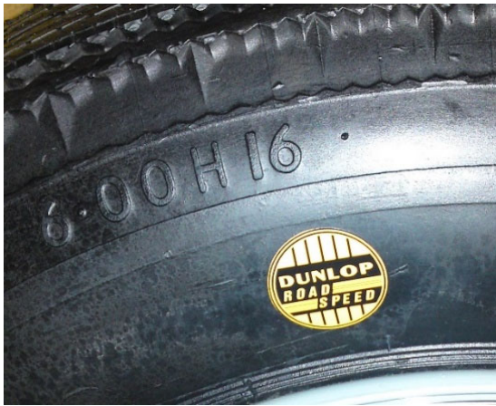
A reproduction DUNLOP RS5 cross-ply Tyre showing its speed-rating 'H' which was introduced from early 1960s onwards, but also showing a correct reproduction DUNLOP decal fitted to many XK 120 original equipment DUNLOP ROADSPEED Tyres. (Photo by Robert Sheridan)
