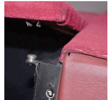
Spring clip, button at sides of parcel box.
