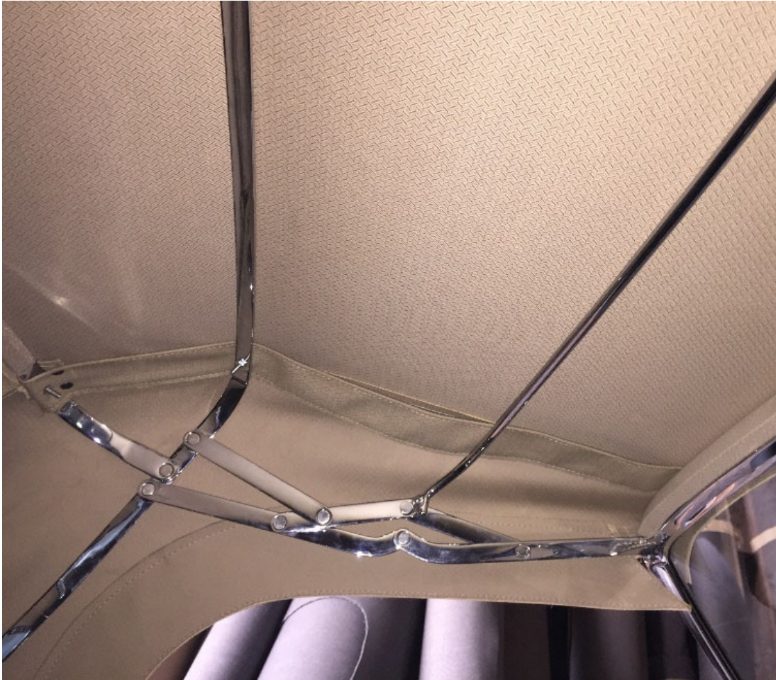
BD.4727 style-2 hoodsticks (metal frame) are chrome-plated and are used with early steel bodied OTS cars until mid-1951.
