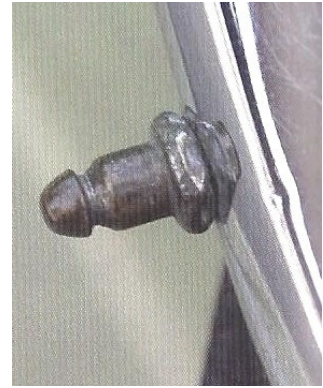
Later front 'Lift-the-dot' stud. (August 1951) onwards.
