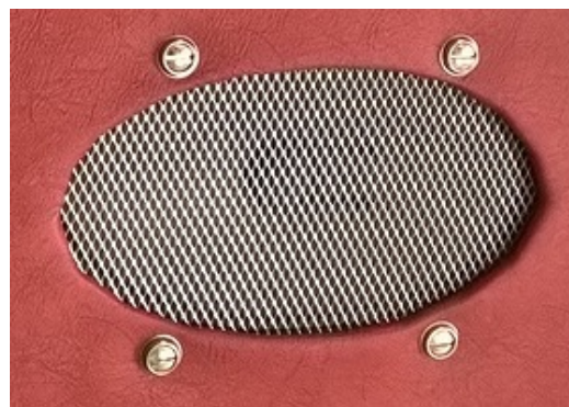
Sample OTS Speaker Mesh, located on the underside of the Passenger Side Scuttle Casing. (Photo by Rob Reilly)
