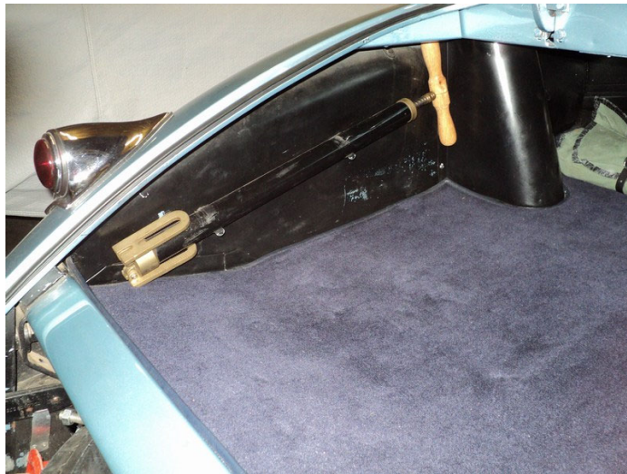
Early steel-bodied cars, until end of 1950, had the tyre pump on left-hand side as pictured above. Early steel-bodied cars, until end of 1950, had the tyre pump clipped onto the left-hand side panel as pictured above. (NOTE, pictured tyre pump with brass feet is a reproduction)
