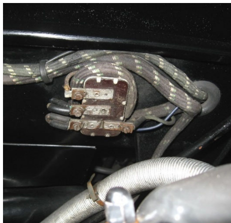
Later steel-bodied car horn relay. (Photo by Robert Sheridan)
