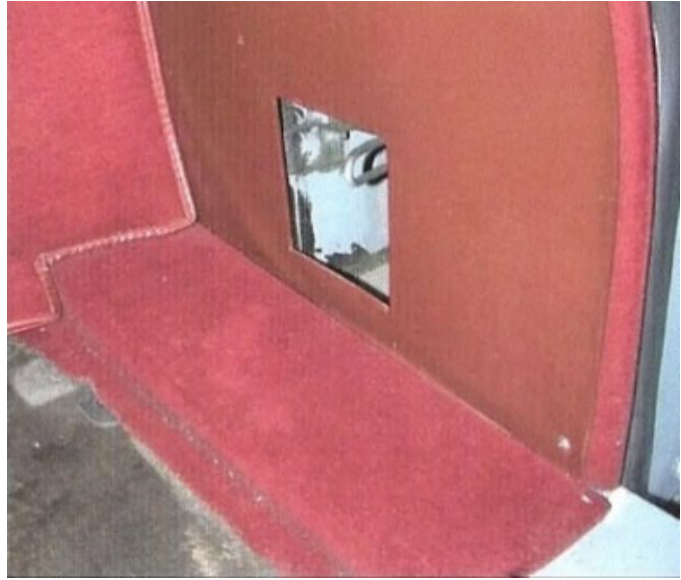
Moquette covered plywood fillet at front of sill near the Footwell.
