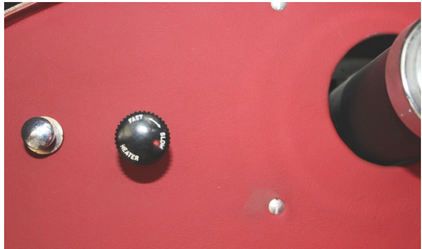
Fog light switch (Lucas 031216) with its knurled chrome-plated knob next to an early heater rheostat knob, correctly located on the driver's side fascia panel. (Photo by Robert Sheridan)
