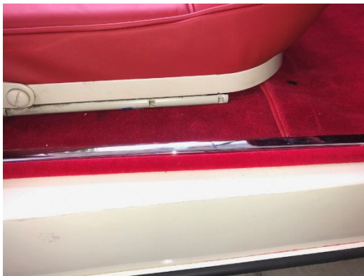
Steel-bodied carpet with chrome carpet rail and draft excluder (Furflex) along the door sill and up each 'A and B' door post. Photo on left by Robert Sheridan. Photo on right © Copyright 2002 by Urs Schmid.
