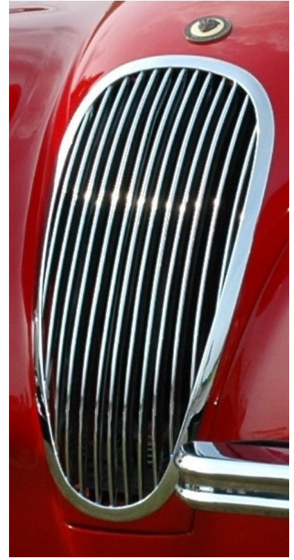
Later grille vanes have rounded leading edges.
