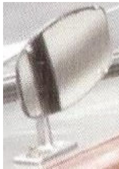
From October 1950 to February 1951 and some later, (C.4645) oval convex glass interior mirror, short stem.
