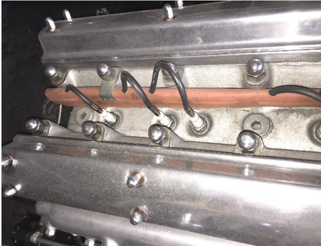
EARLY ignition wires entering a terracotta colored fiberboard conduit from the back of the head, until Engine No. W.6696. (NOTE: the plain metal terminals and conduit bracket on second stud from the rear).
