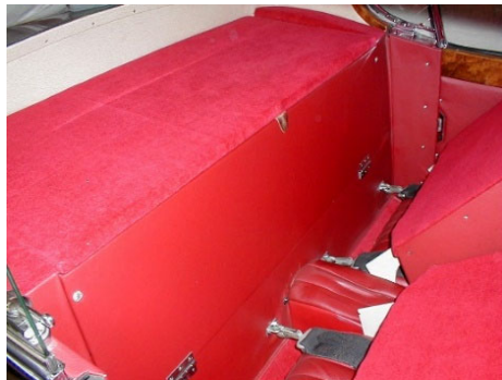
View of parcel box assembly closed. Note leather pull strap at top and two hinges below. Parcel box lid covered in carpet.
