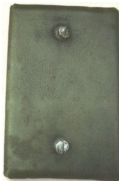
Transmission dipstick cover with 2 Oddie stud fasteners. (Photo on left by Robert Sheridan. Photos on the right © Copyright 2002 by Urs Schmid)
