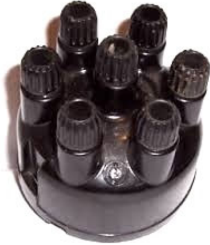
Later Distributor Cover from February 1953 onwards, with vertical high-tension lead outlets, with seven fluted Bakelite nuts to secure the high-tension leads.
