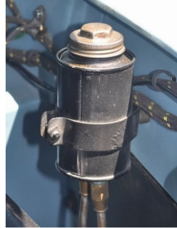
Brake supply tank including cadmium-plated filler cap.
