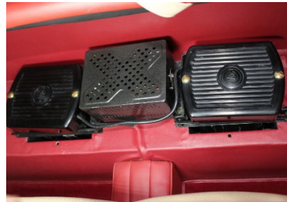
View of the Batteries covered with Lucas cover plates. (Photos above by Robert Sheridan)
