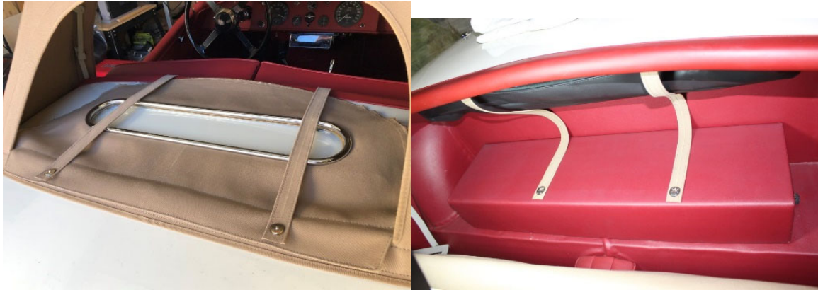
Views of the two canvas straps used to hold BD.5866 style-2 hood backlight in place when folded down. (Photos by Robert Sheridan)
