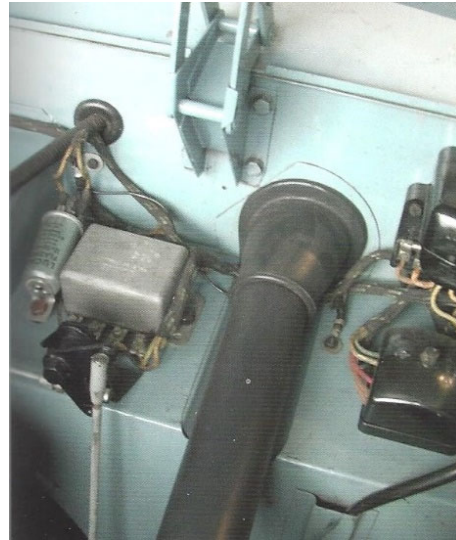
FHC/DHC steering column rubber grommet. (Photo © copyright 2002 by Urs Schmid) NOTE: Refer to rubber grommet only.
