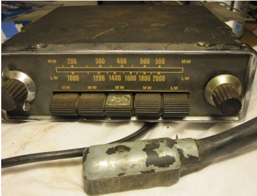
Early C.4063 car radio assembly Radiomobile model RP.100, with 'His Master's Voice' on the middle button.
