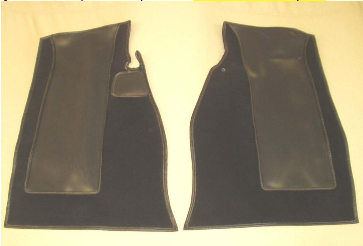
Photo of front carpet set for OTS and FHC showing vinyl inserts by Chuck Diamond
